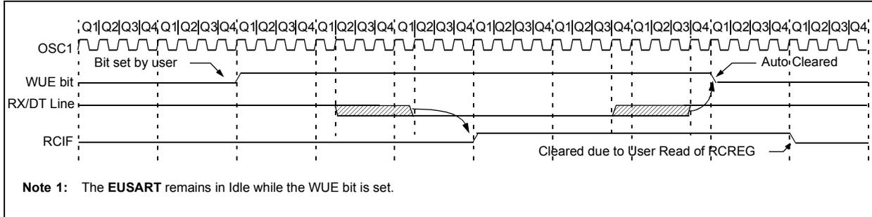
**FIGURE 29-8: AUTO-WAKE-UP BIT (WUE) TIMINGS DURING SLEEP**
