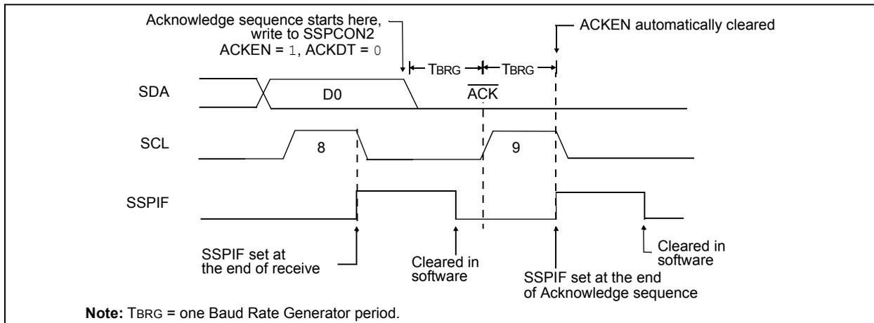
**FIGURE 28-31: STOP CONDITION RECEIVE OR TRANSMIT MODE**
