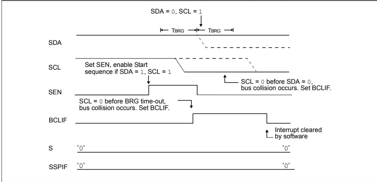
**FIGURE 28-35: BRG RESET DUE TO SDA ARBITRATION DURING START CONDITION**
