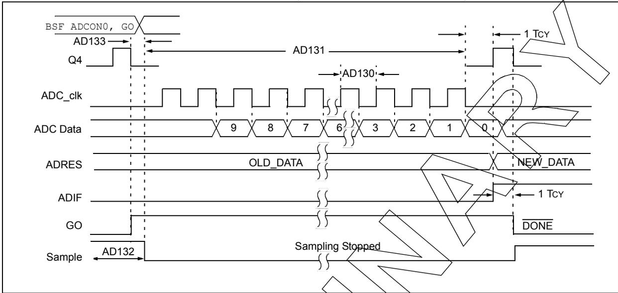
**FIGURE 32-14: ADC CONVERSION TIMING (ADC CLOCK FROM FRC)**
