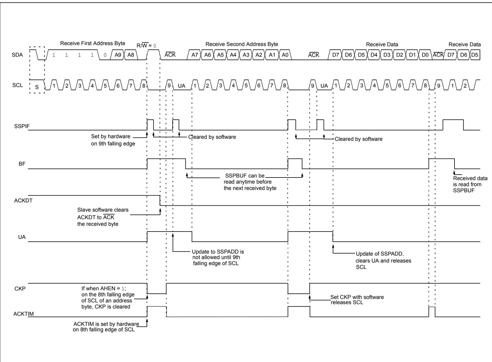
FIGURE 28-22: I<sup>2</sup>C SLAVE, 10-BIT ADDRESS, TRANSMISSION (SEN = 0, AHEN = 0, DHEN = 0)
