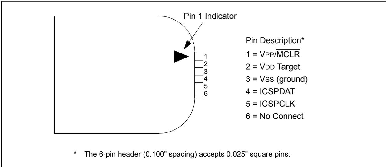
**FIGURE 30-3: TYPICAL CONNECTION FOR ICSP™ PROGRAMMING**
