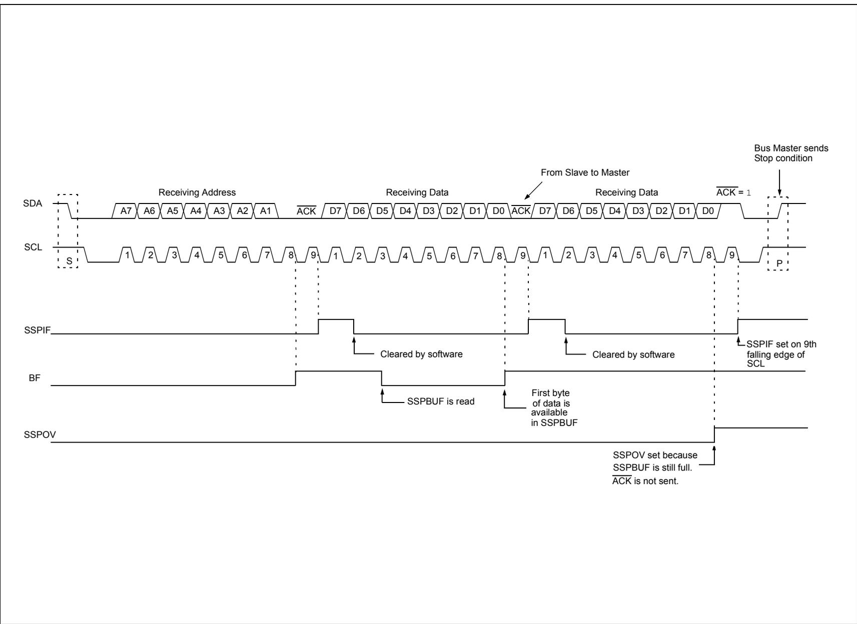
FIGURE 28-15: I<sup>2</sup>C SLAVE, 7-BIT ADDRESS, RECEPTION (SEN = 1, AHEN = 0, DHEN = 0)
