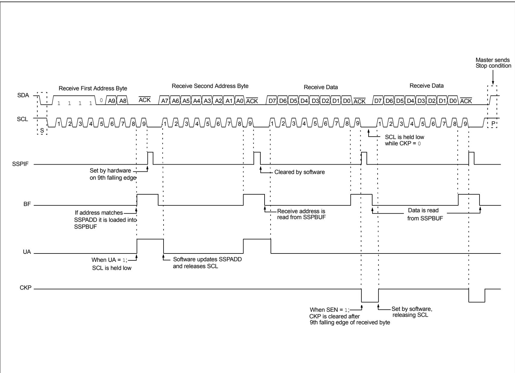
FIGURE 28-21: I<sup>2</sup>C SLAVE, 10-BIT ADDRESS, RECEPTION (SEN = 0, AHEN = 1, DHEN = 0)
