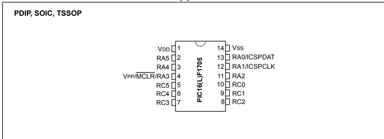
**FIGURE 2: 16-PIN PACKAGE DIAGRAM FOR PIC16(L)F1705**
