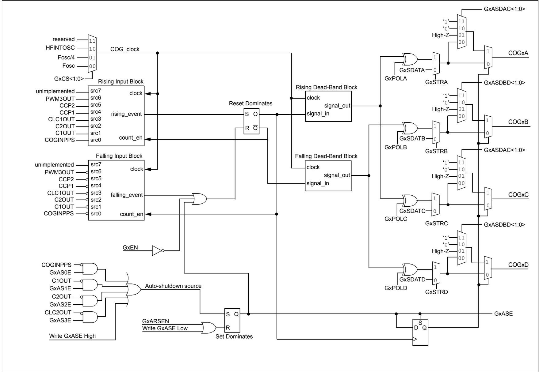
**FIGURE 18-6: SIMPLIFIED COG BLOCK DIAGRAM (PUSH-PULL MODE, GXMD = 5)**
