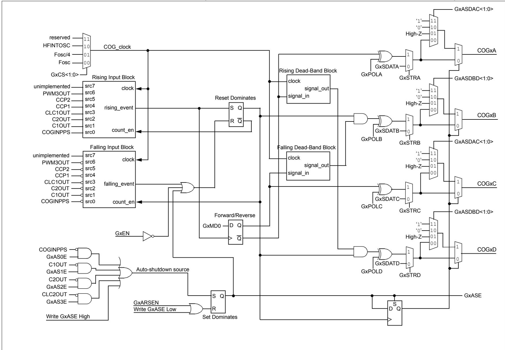
FIGURE 18-5: SIMPLIFIED COG BLOCK DIAGRAM (HALF-BRIDGE MODE, GXMD = 4)
