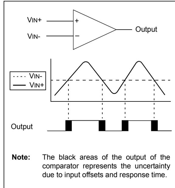
**FIGURE 16-2: COMPARATOR MODULE SIMPLIFIED BLOCK DIAGRAM**
