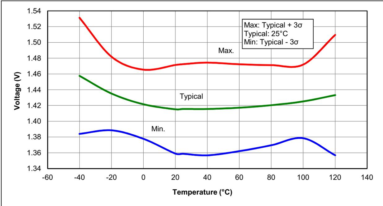
**FIGURE 33-9: BROWN-OUT RESET VOLTAGE, BORV = 1, PIC16LF1705/9 ONLY**
