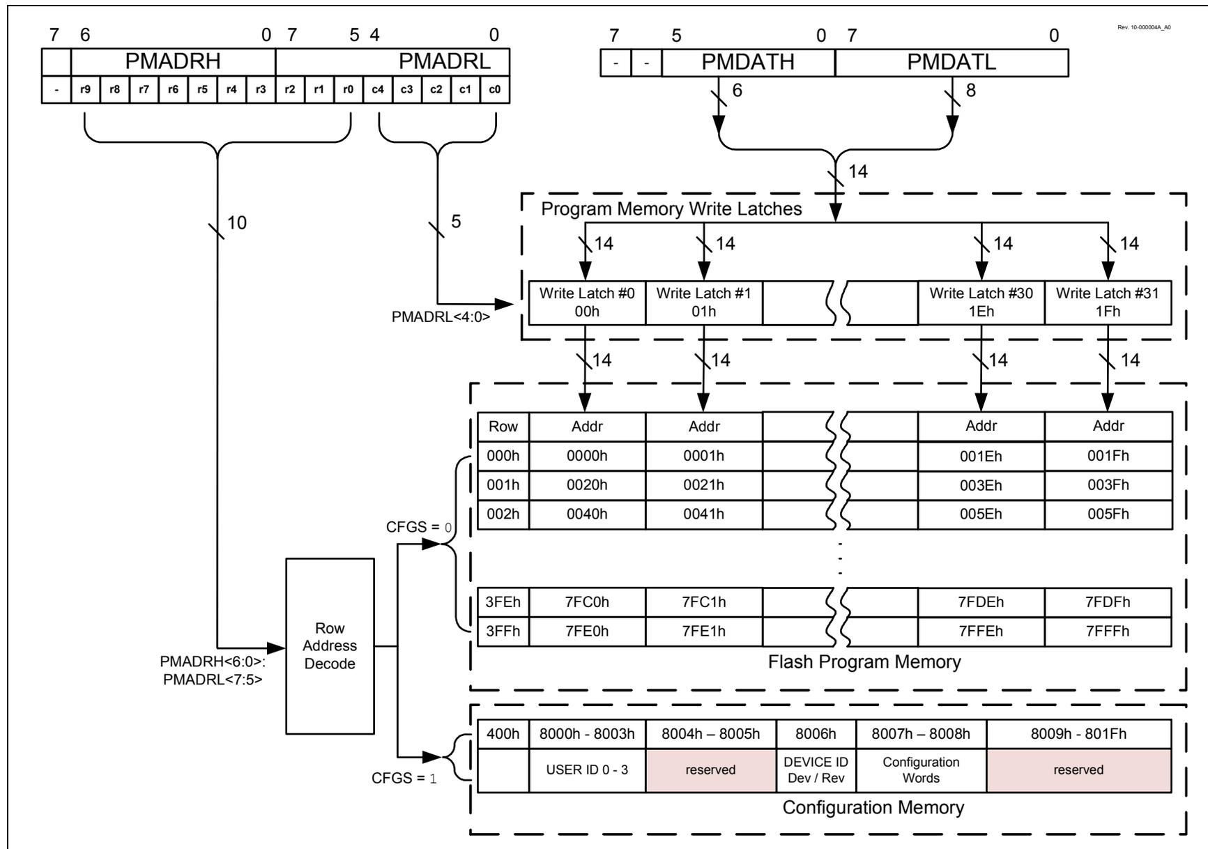
**FIGURE 10-6: FLASH PROGRAM MEMORY WRITE FLOWCHART**
