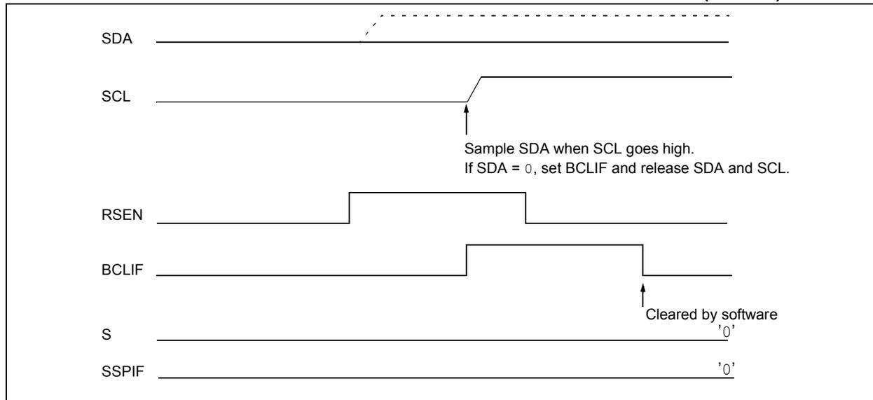
**FIGURE 28-37: BUS COLLISION DURING REPEATED START CONDITION (CASE 2)**
