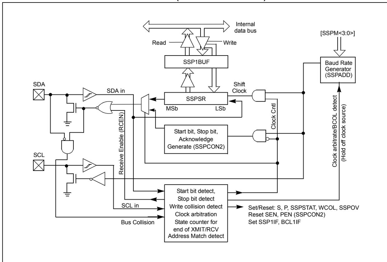
**FIGURE 28-3: MSSP BLOCK DIAGRAM (I<sup>2</sup>C™ SLAVE MODE)**
