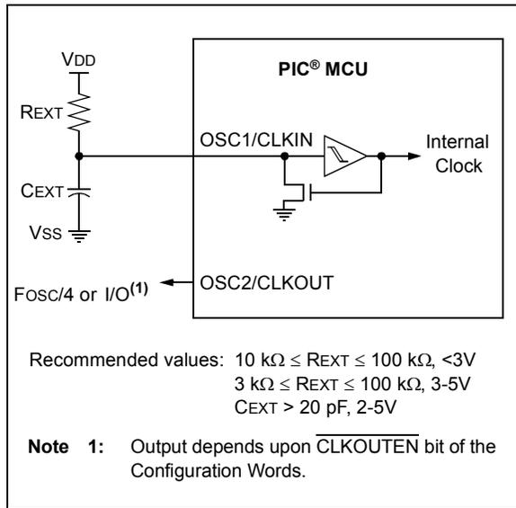
The RC oscillator frequency is a function of the supply voltage, the resistor ( $R_{EXT}$ ) and capacitor ( $C_{EXT}$ ) values and the operating temperature. Other factors affecting the oscillator frequency are:
