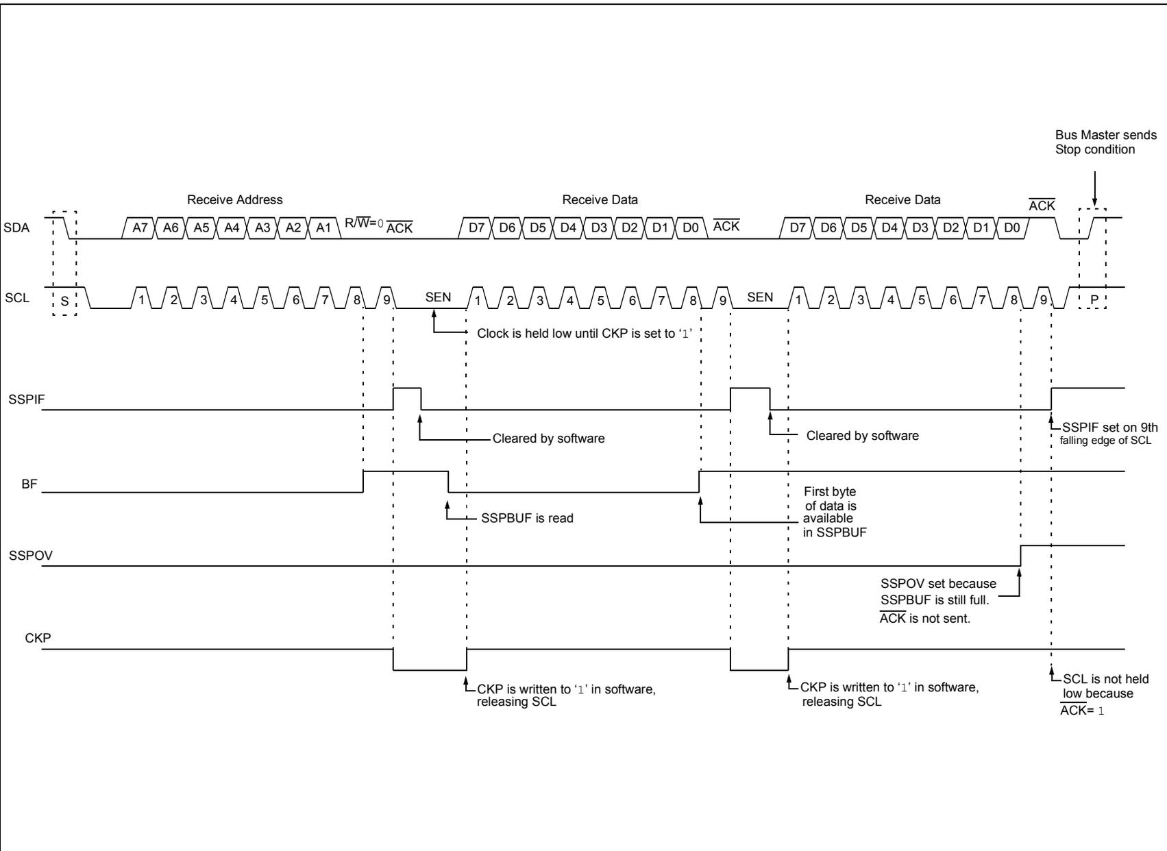
FIGURE 28-16: I<sup>2</sup>C SLAVE, 7-BIT ADDRESS, RECEPTION (SEN = 0, AHEN = 1, DHEN = 1)
