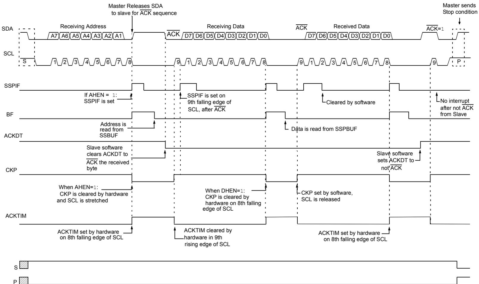
FIGURE 28-17: I<sup>2</sup>C SLAVE, 7-BIT ADDRESS, RECEPTION (SEN = 1, AHEN = 1, DHEN = 1)
