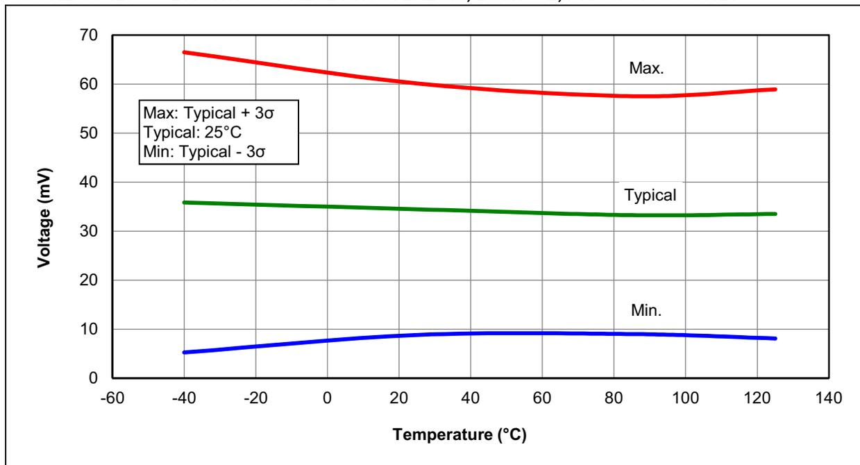
**FIGURE 33-13: BROWN-OUT RESET VOLTAGE, BORV = 0**
