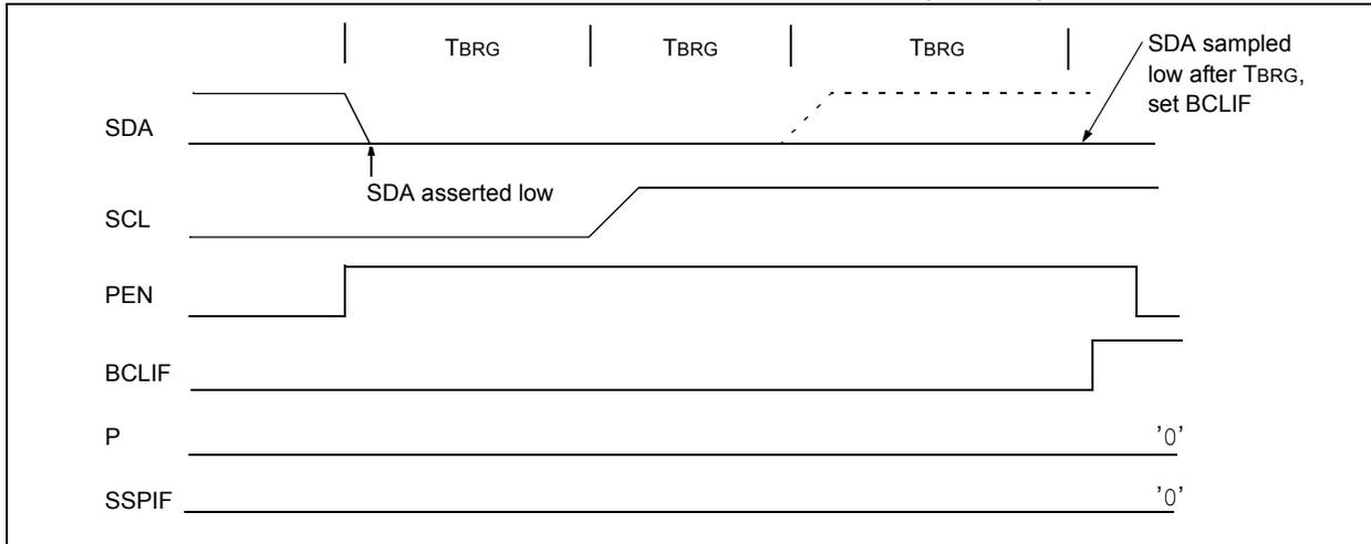
**FIGURE 28-39: BUS COLLISION DURING A STOP CONDITION (CASE 2)**
