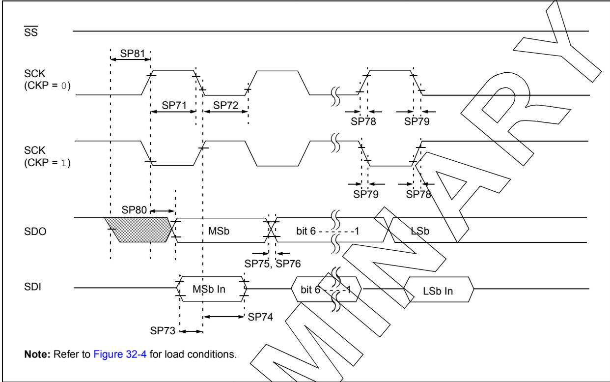
**FIGURE 32-18: SPI MASTER MODE TIMING (CKE = 1, SMP = 1)**
