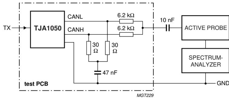
Fig.8 Basic test set-up (with split termination) for electromagnetic emission measurement (see Figs 9 and 10).
