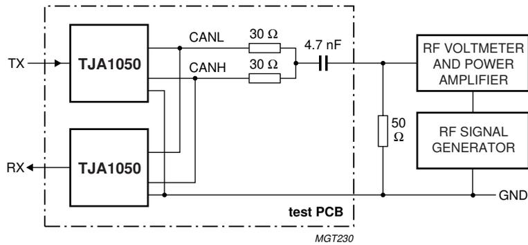
Fig.11 Basic test set-up for electromagnetic immunity measurement (see Fig.12).
