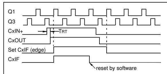
**FIGURE 20-5: COMPARATOR INTERRUPT TIMING WITH CMxCON0 READ**
