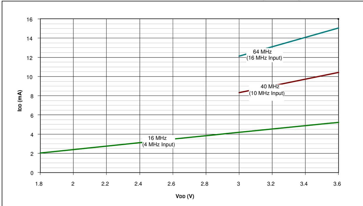
FIGURE 27-14: PIC18F4XK20/PIC18F2XK20 MAXIMUM PRI\_RUN IDD (HS + PLL)
