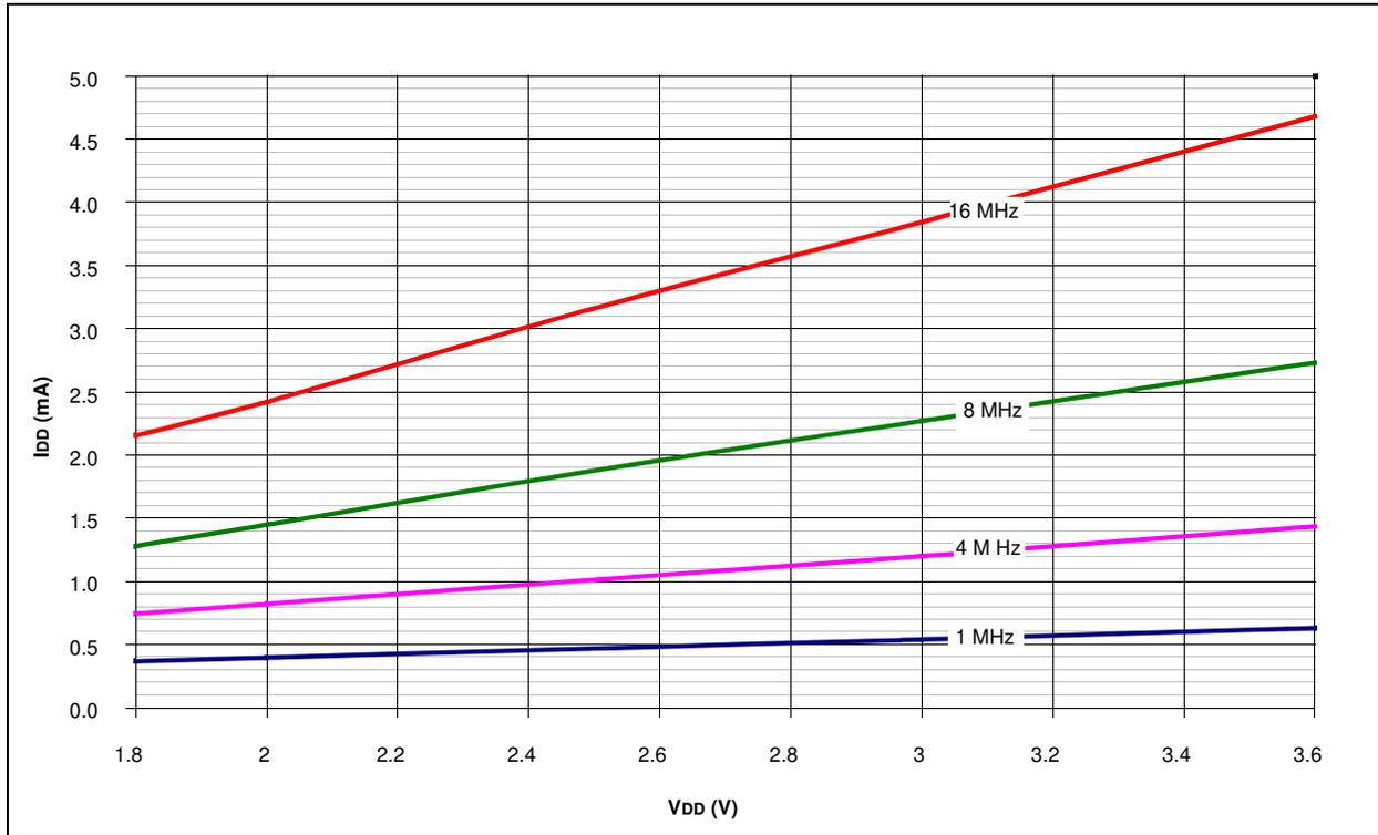
FIGURE 27-6: PIC18F4XK20/PIC18F2XK20 MAXIMUM RC\_RUN IDD
