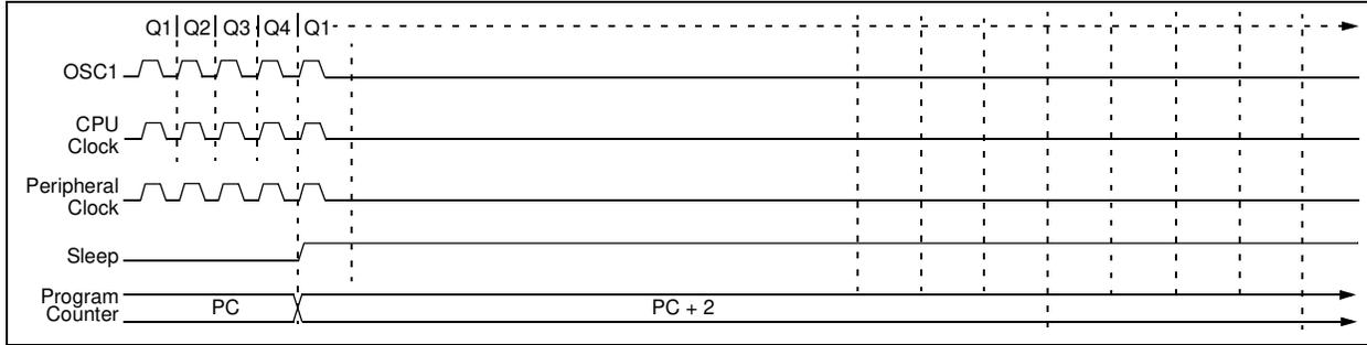
**FIGURE 3-2: TRANSITION TIMING FOR WAKE FROM SLEEP (HSPLL)**
