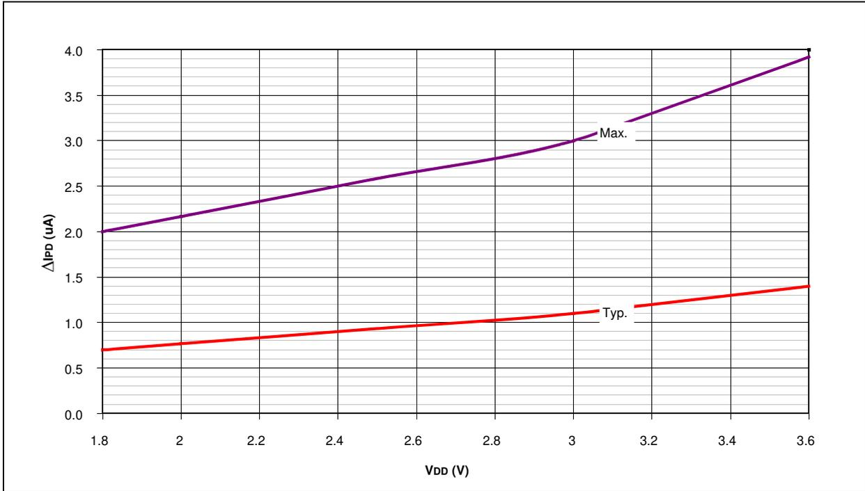
**FIGURE 27-18: PIC18F4XK20/PIC18F2XK20  $\Delta I_{BOR}$  and  $\Delta I_{HLVD}$  – Delta IPD for Brown-out Reset and High/Low Voltage Detect, -40°C to +125°C**
