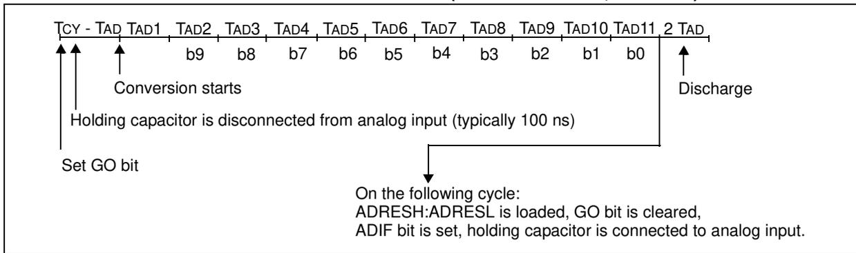
**FIGURE 19-4: A/D CONVERSION TAD CYCLES (`ACQT<2:0> = 010, TACQ = 4 TAD`)**
