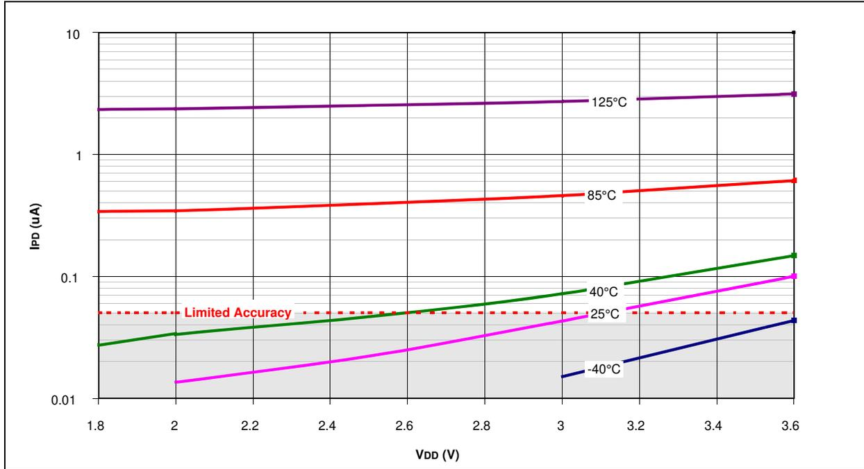
FIGURE 27-2: PIC184XK20/PIC18F2XK20 MAXIMUM BASE IPD
