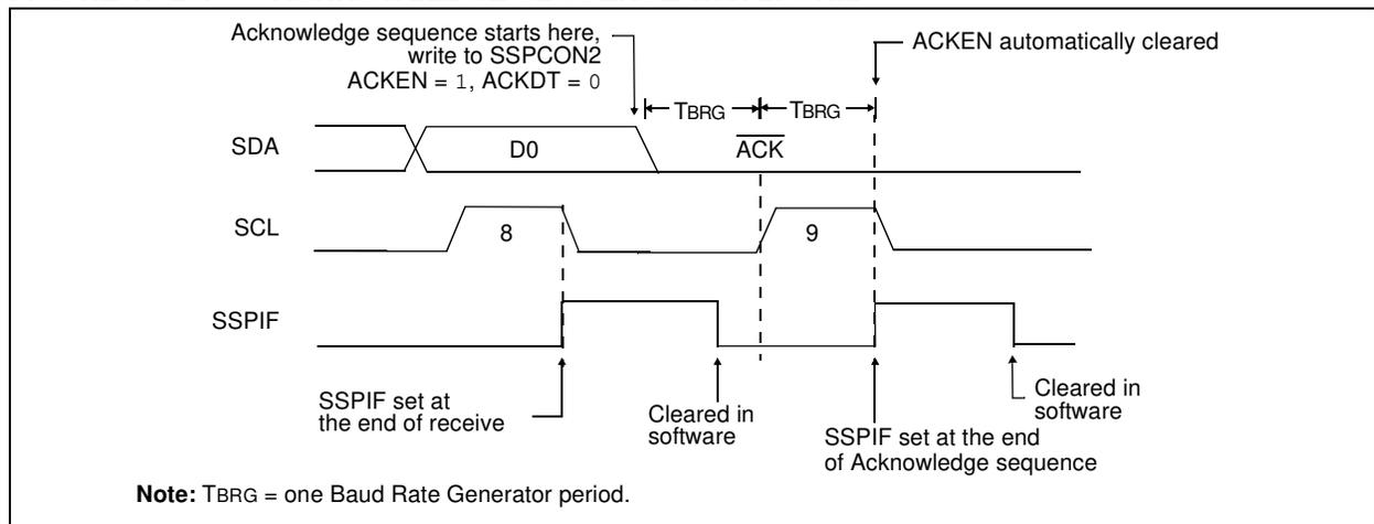
**FIGURE 17-24: STOP CONDITION RECEIVE OR TRANSMIT MODE**
