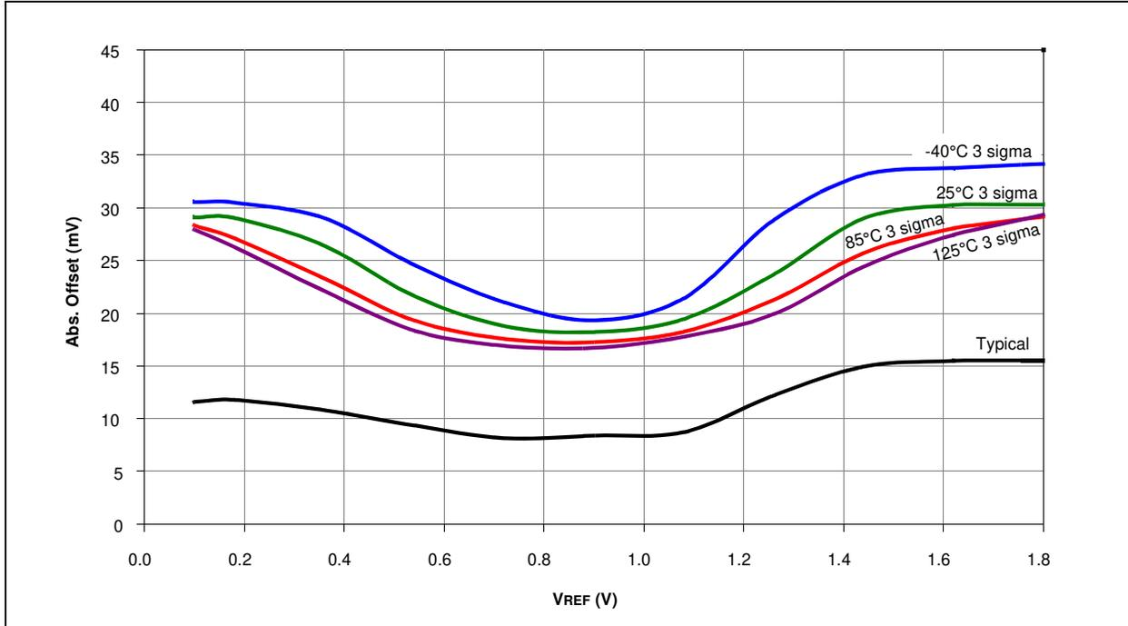
FIGURE 27-32: PIC18F4XK20/PIC18F2XK20 COMPARATOR OFFSET (HIGH POWER,  $V_{DD} = 3.6V$ )
