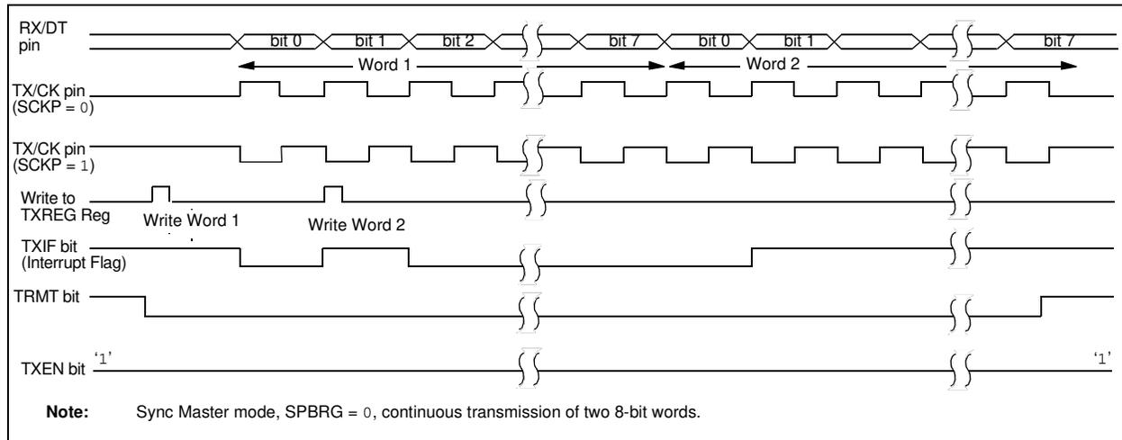
**FIGURE 18-11: SYNCHRONOUS TRANSMISSION (THROUGH TXEN)**
