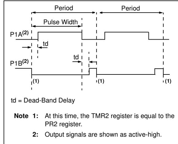
**FIGURE 16-13: EXAMPLE OF HALF-BRIDGE APPLICATIONS**
