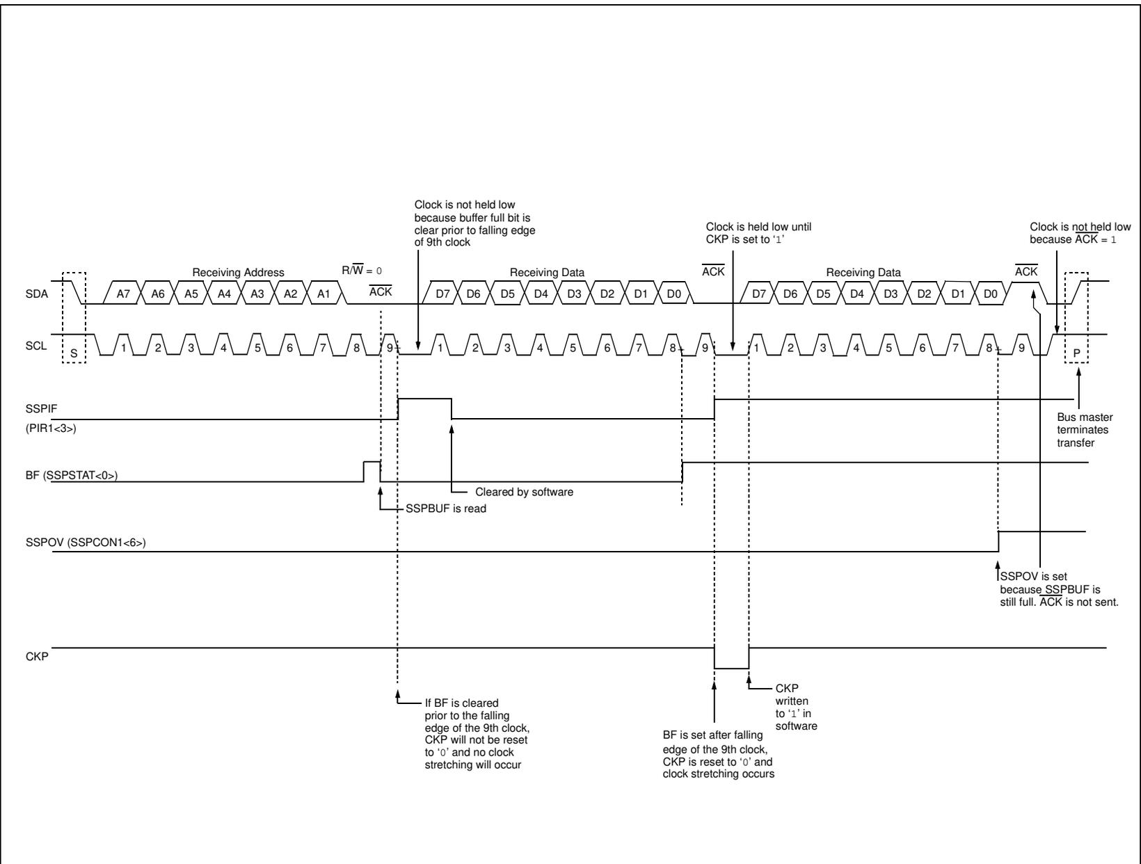
FIGURE 17-14: I<sup>2</sup>C™ SLAVE MODE TIMING WITH SEN = 1 (RECEPTION, 10-BIT ADDRESS)
