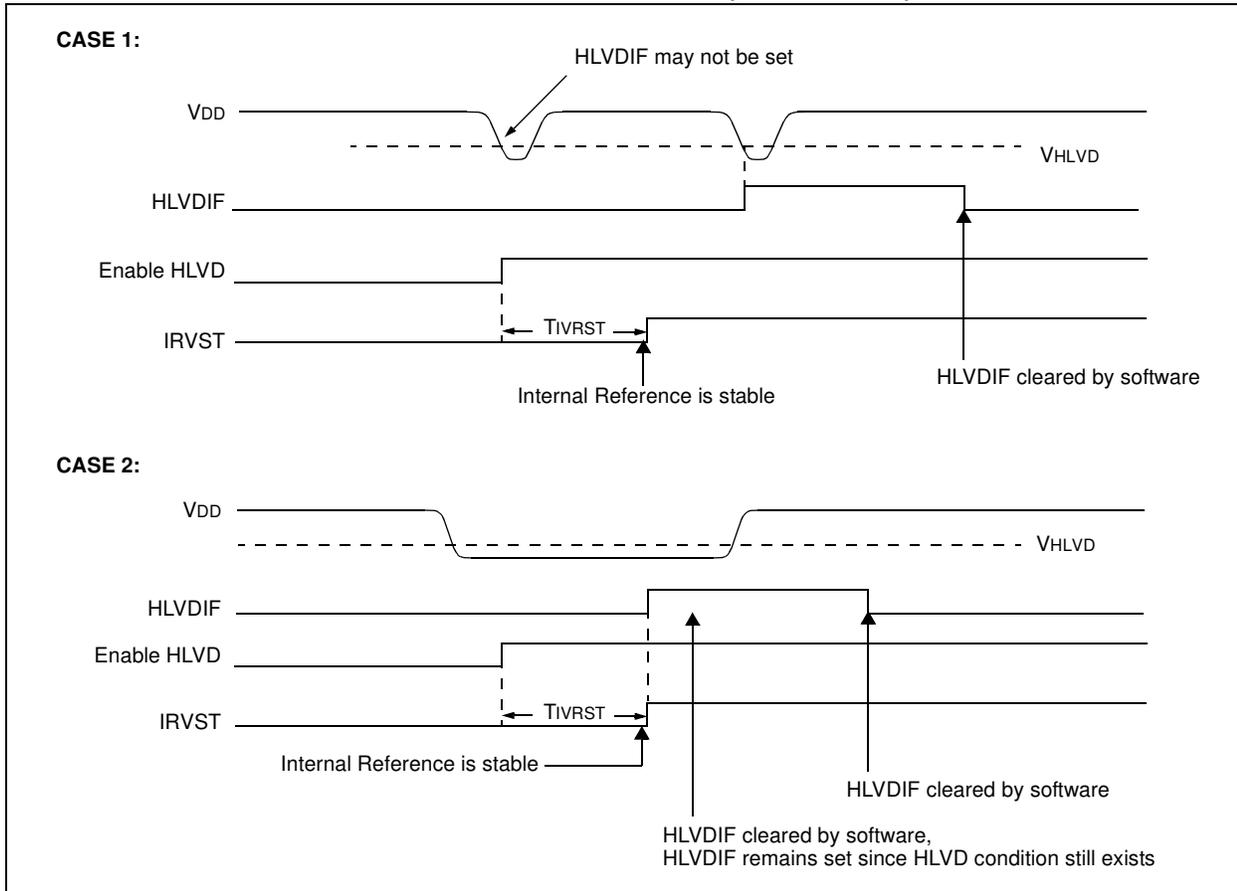
**FIGURE 22-3: HIGH-VOLTAGE DETECT OPERATION (VDIRMAG = 1)**
