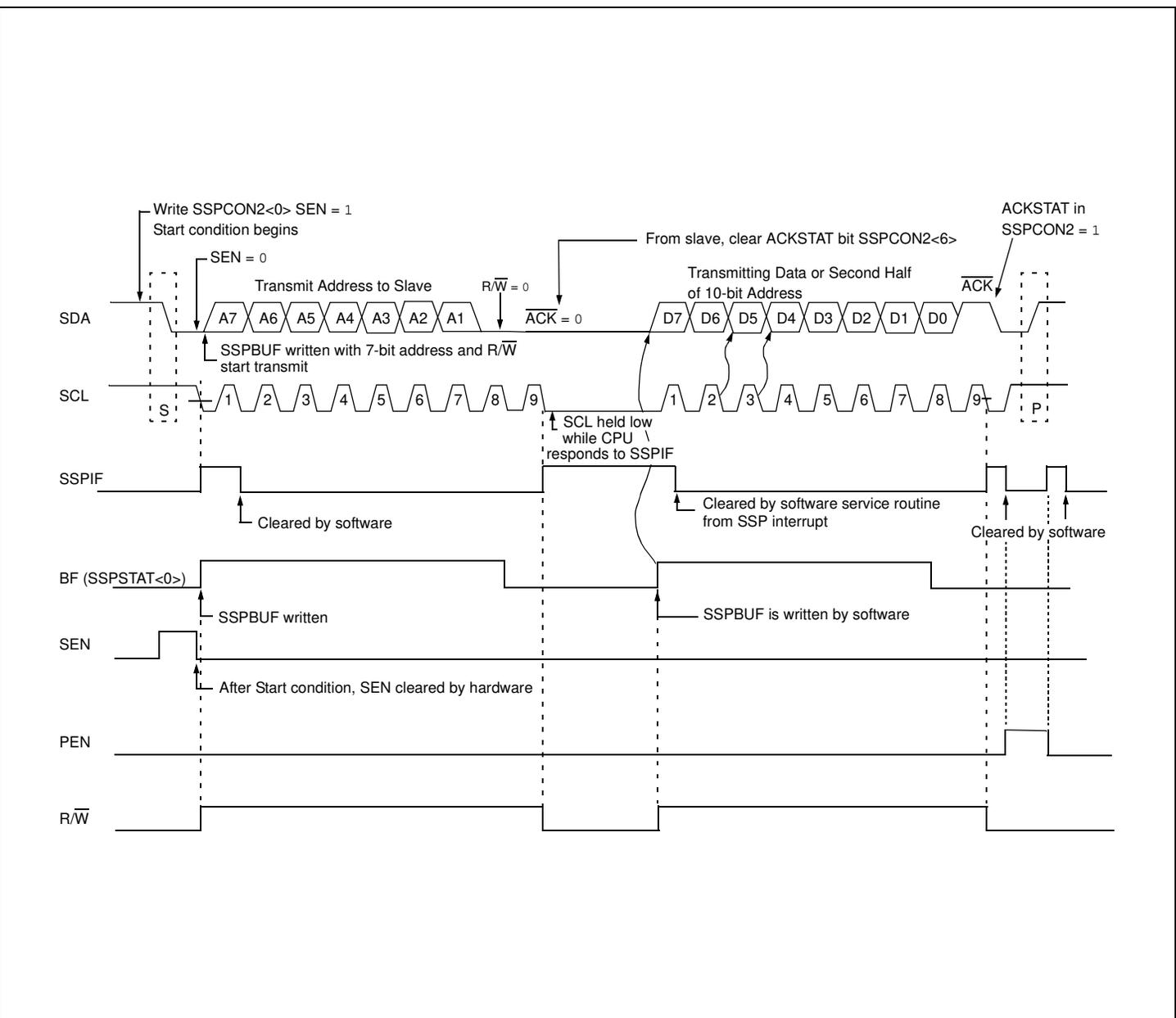
FIGURE 17-22: I<sup>2</sup>C™ MASTER MODE WAVEFORM (RECEPTION, 7-BIT ADDRESS)
