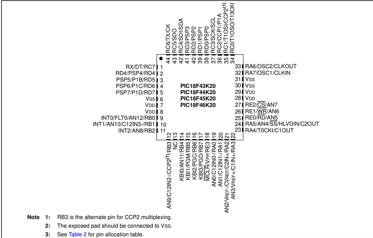
**FIGURE 6: 44-PIN TQFP**
