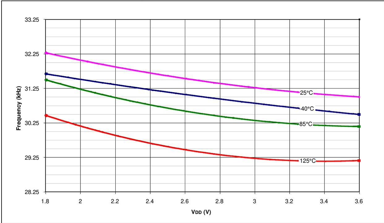
**FIGURE 27-45: PIC18F4XK20/PIC18F2XK20 TYPICAL LF-INTOSC FREQUENCY (MAX./MIN. = 31.25 kHz +/-15%)**
