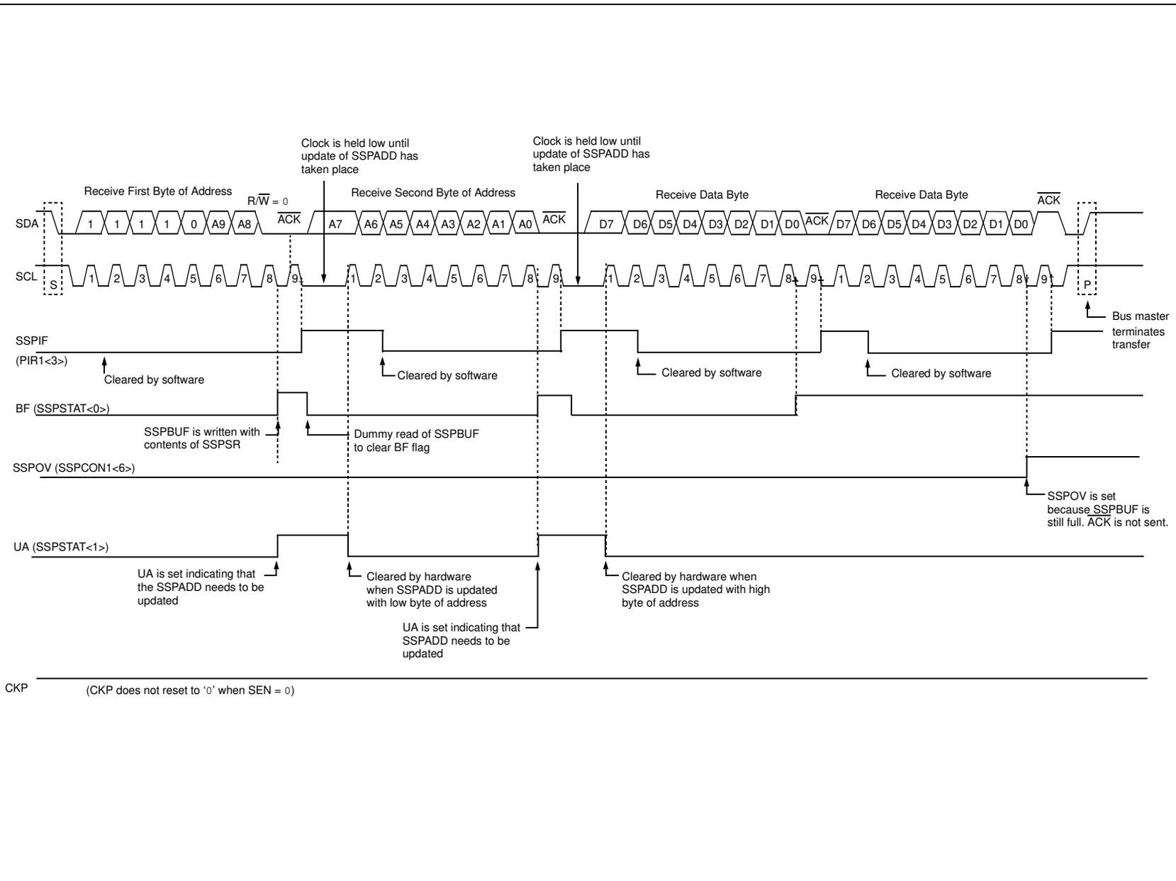
FIGURE 17-11: I<sup>2</sup>C™ SLAVE MODE TIMING (TRANSMISSION, 10-BIT ADDRESS)
