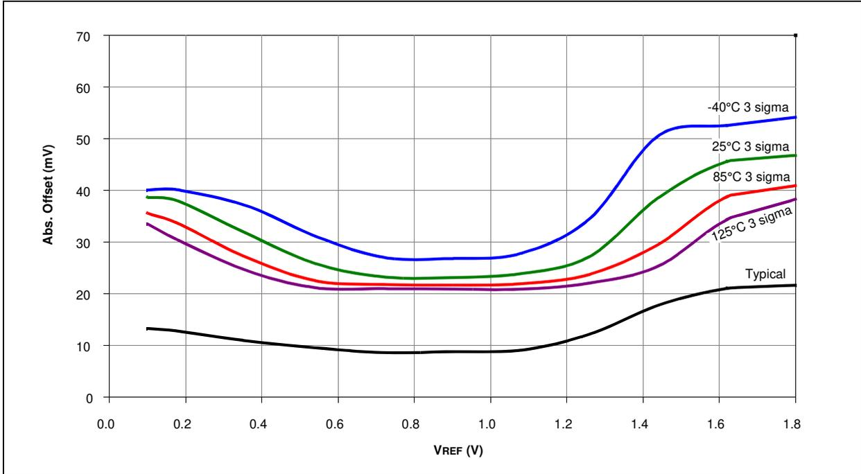
FIGURE 27-30: PIC18F4XK20/PIC18F2XK20 COMPARATOR OFFSET (LOW POWER,  $V_{DD} = 3.6V$ )
