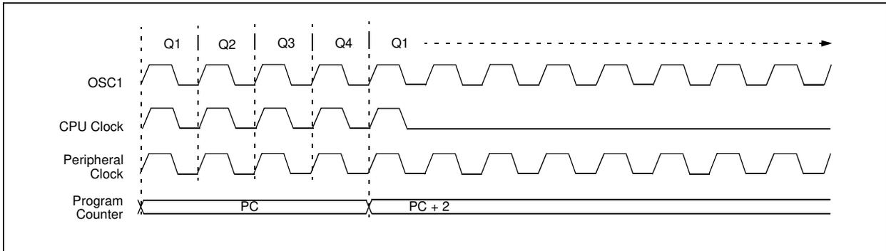
**FIGURE 3-4: TRANSITION TIMING FOR WAKE FROM IDLE TO RUN MODE**
