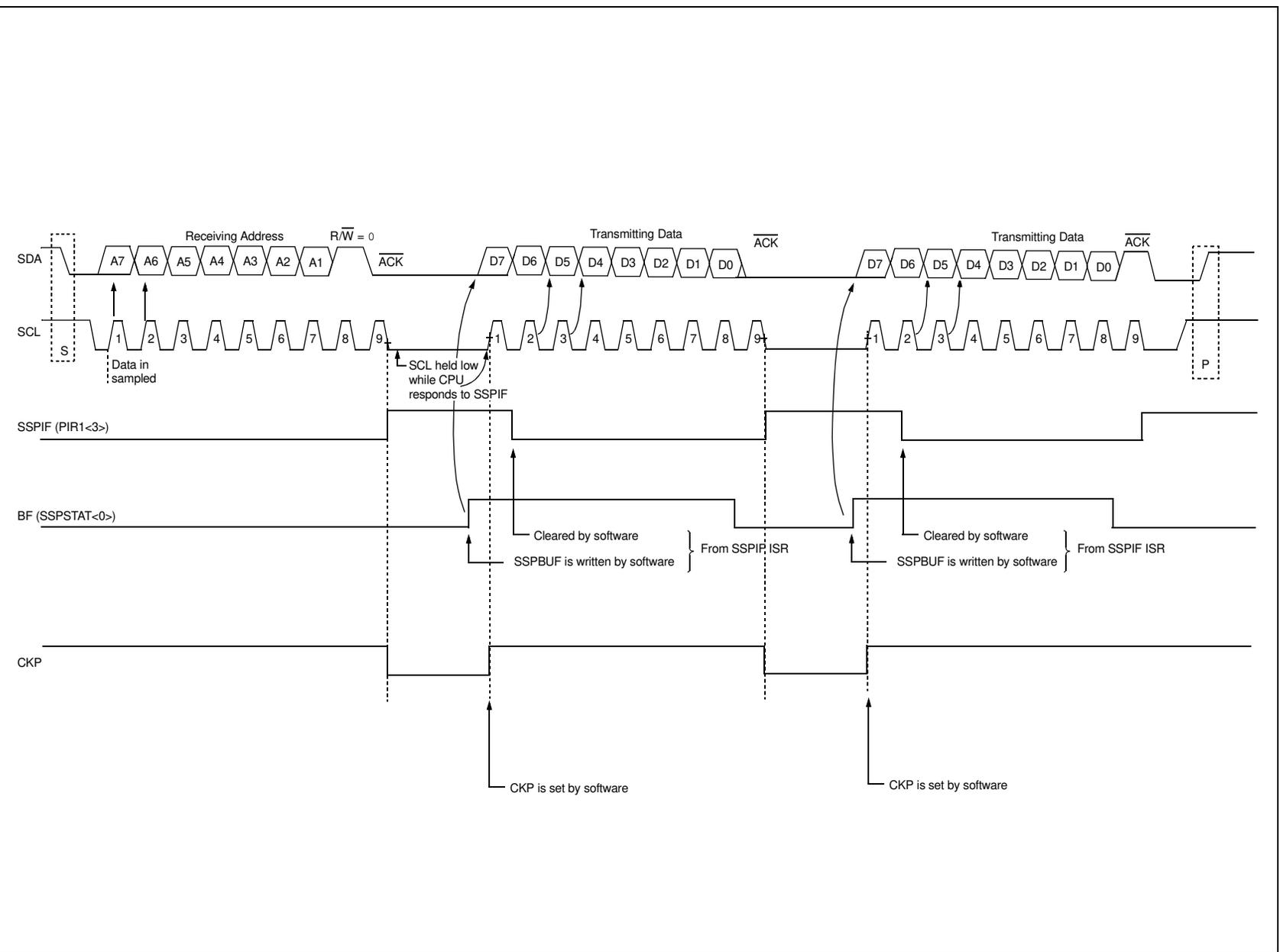
FIGURE 17-10: I<sup>2</sup>C™ SLAVE MODE TIMING WITH SEN = 0 (RECEPTION, 10-BIT ADDRESS)
