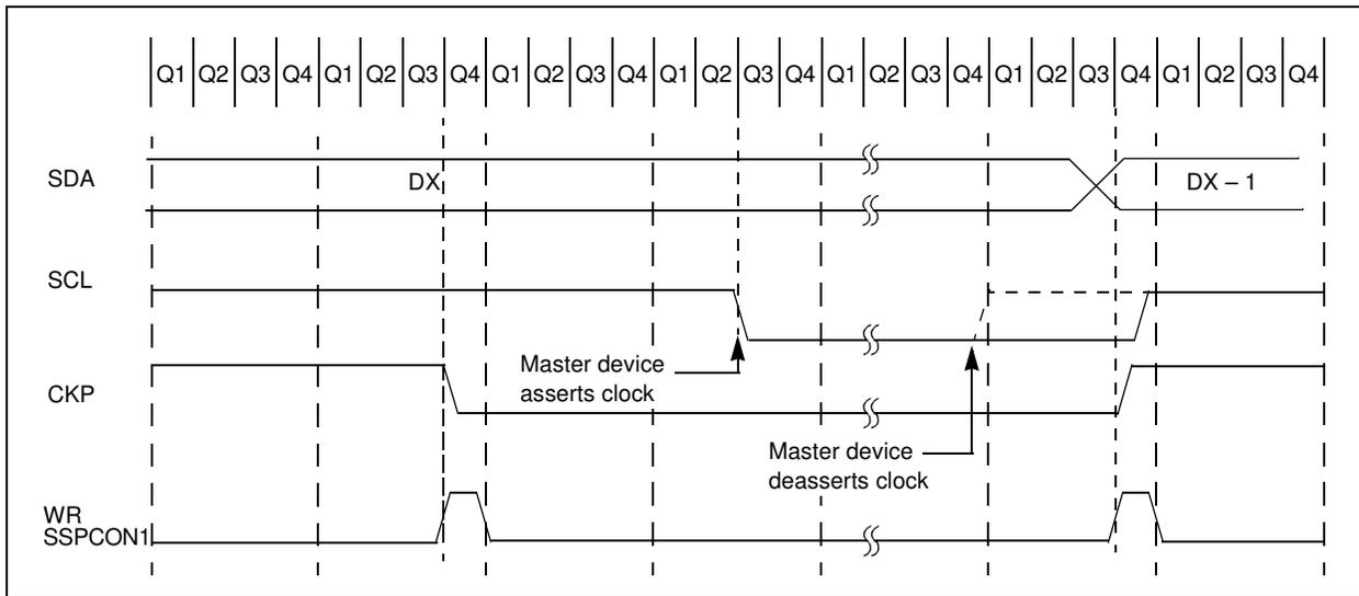
FIGURE 17-13: I<sup>2</sup>C™ SLAVE MODE TIMING WITH SEN = 1 (RECEPTION, 7-BIT ADDRESS)
