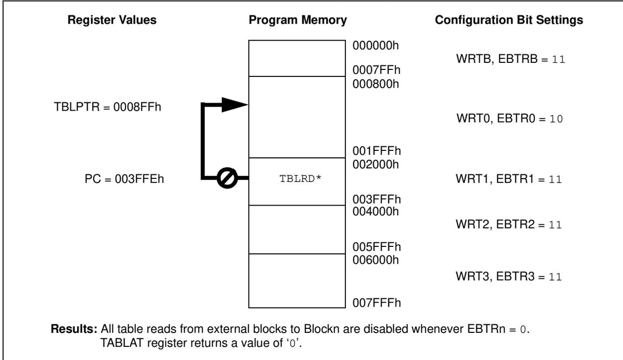
**FIGURE 23-5: EXTERNAL BLOCK TABLE READ (EBTRn) ALLOWED**
