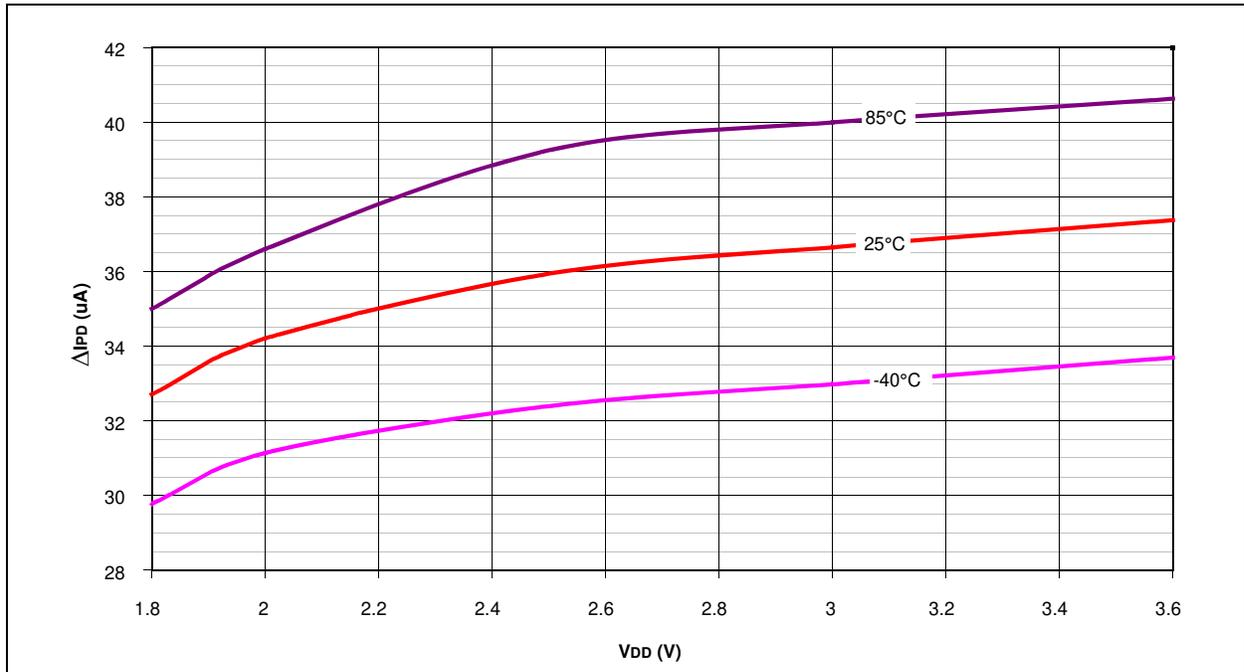
**FIGURE 27-22: PIC18F4XK20/PIC18F2XK20  $\Delta I_{CVREF}$  – Delta IPD for Comparator Voltage Reference, -40°C to +125°C**
