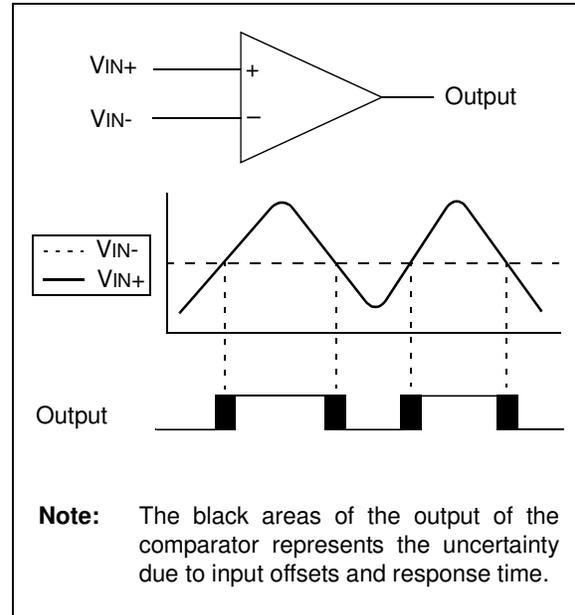
**FIGURE 20-2: COMPARATOR C1 SIMPLIFIED BLOCK DIAGRAM**
