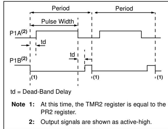
**FIGURE 16-5: EXAMPLE OF HALF-BRIDGE APPLICATIONS**
