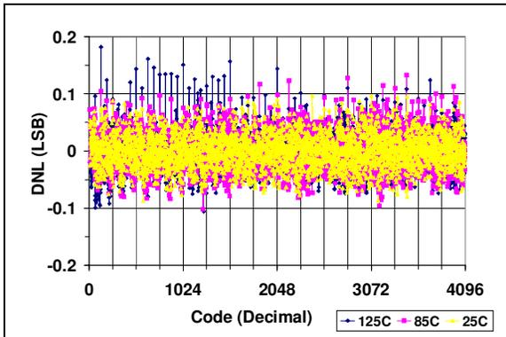
**FIGURE 2-2:** DNL vs. Code and Temperature (MCP4822).
