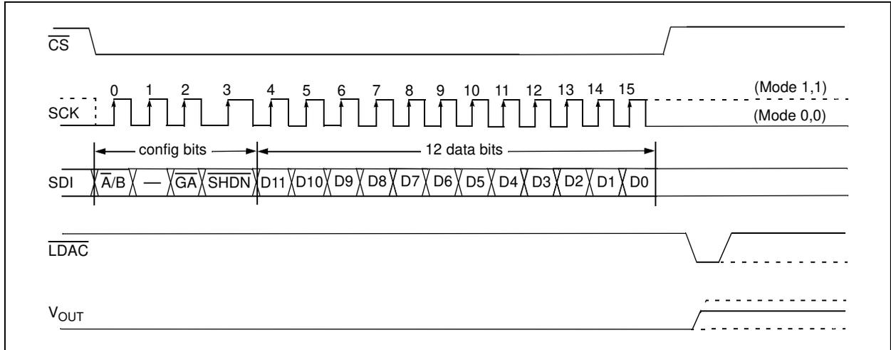
**FIGURE 5-1:** Write Command for MCP4822 (12-bit DAC).
