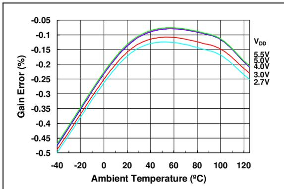
**FIGURE 2-20:** Gain Error vs. Temperature and  $V_{DD}$ .
