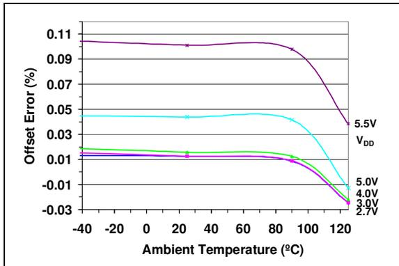
**FIGURE 2-19:** Offset Error vs. Temperature and  $V_{DD}$ .
