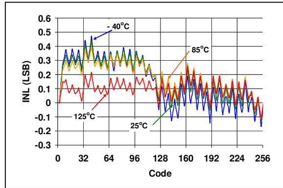
**FIGURE 2-10:** INL vs. Code and Temperature (MCP4802).
