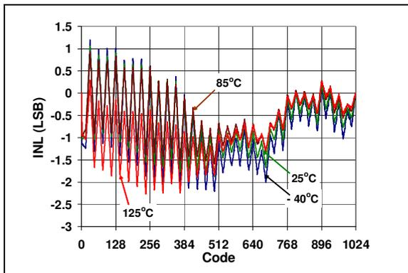
**FIGURE 2-8:** INL vs. Code and Temperature (MCP4812).
