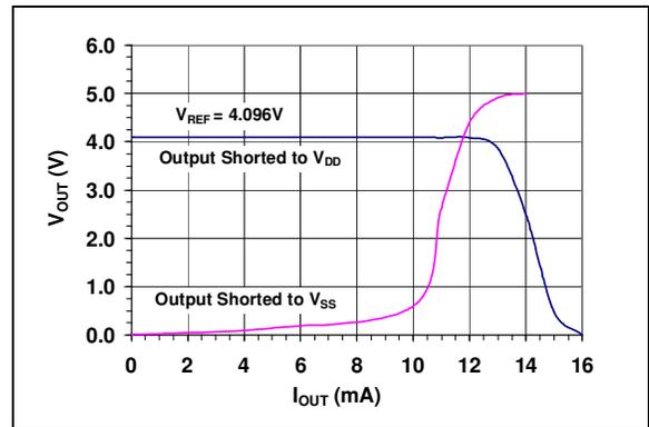
**FIGURE 2-27:**  $I_{OUT}$  vs.  $V_{OUT}$ .  $\text{Gain} = 2x$ .
