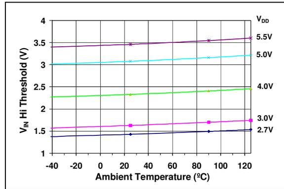
**FIGURE 2-21:**  $V_{IN}$  High Threshold vs. Temperature and  $V_{DD}$ .
