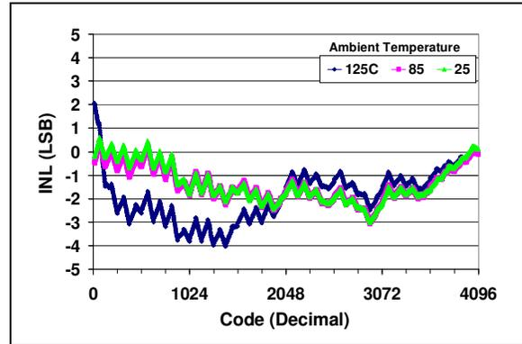
**FIGURE 2-4:** INL vs. Code and Temperature (MCP4822).
