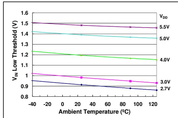
**FIGURE 2-22:**  $V_{IN}$  Low Threshold vs. Temperature and  $V_{DD}$ .
