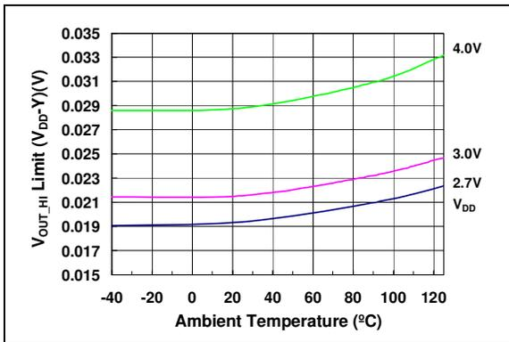
**FIGURE 2-24:**  $V_{OUT}$  High Limit vs. Temperature and  $V_{DD}$ .
