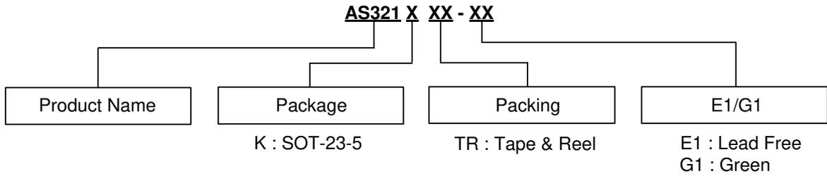
Diodes IC's Pb-free products, as designated with "E1" suffix in the part number, are RoHS compliant.
