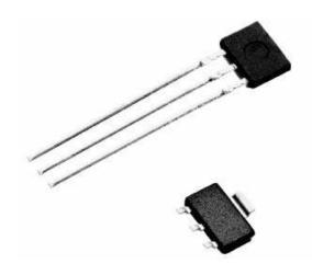
The SS49E and SS59ET Series Economical Linear Hall-effect sensors are small, versatile linear Hall-effect devices that are operated by the magnetic field from a permanent magnet or an electromagnet. The linear sourcing output voltage is set by the supply voltage and varies in proportion to the strength of the magnetic field.
