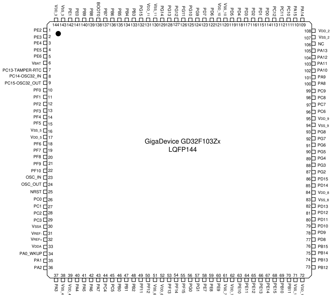
Figure 3. GD32F103Zx LQFP144 pinouts
