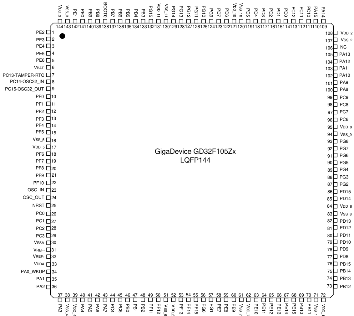
Figure 2. GD32F105Zx LQFP144 pinouts
