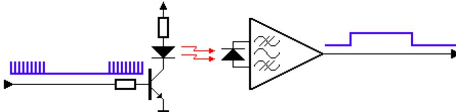
Infrared emitting diode launch out the modulation signal and infrared receiver head will receive, decode, filter and so on to regain the signal .
