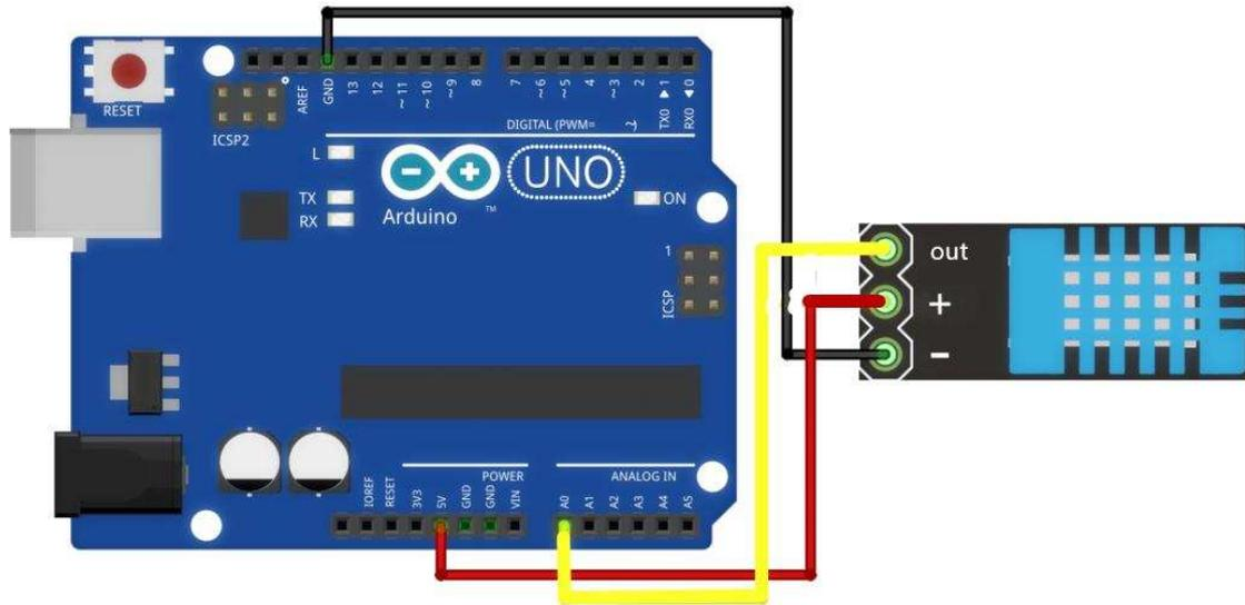
As you can see we only need 3 connections to the sensor, since one of the pin is not used. The connection are : Voltage, Ground and Signal which can be connected to any Analog Pin on our UNO.
