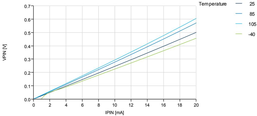
Figure 37-33.I/O Pin Output Voltage vs. Sink Current
