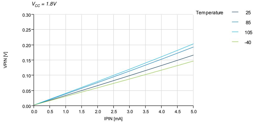
**Figure 37-31. I/O Pin Output Voltage vs. Sink Current**
