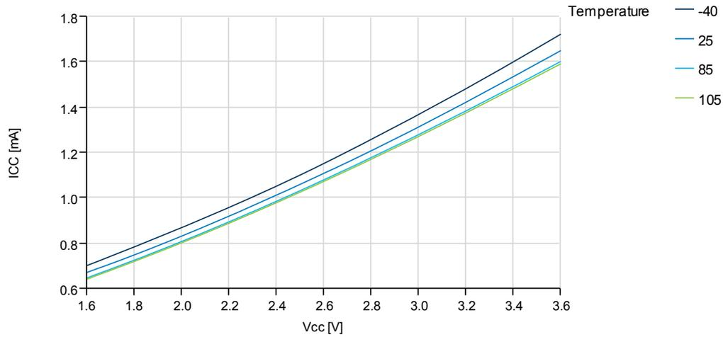
**Figure 37-16. Idle Mode Supply Current vs. V<sub>CC</sub>**
