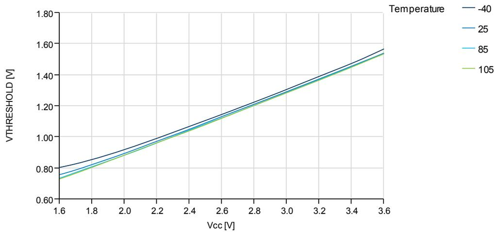
Figure 37-37. I/O Pin Input Hysteresis vs.  $V_{CC}$
