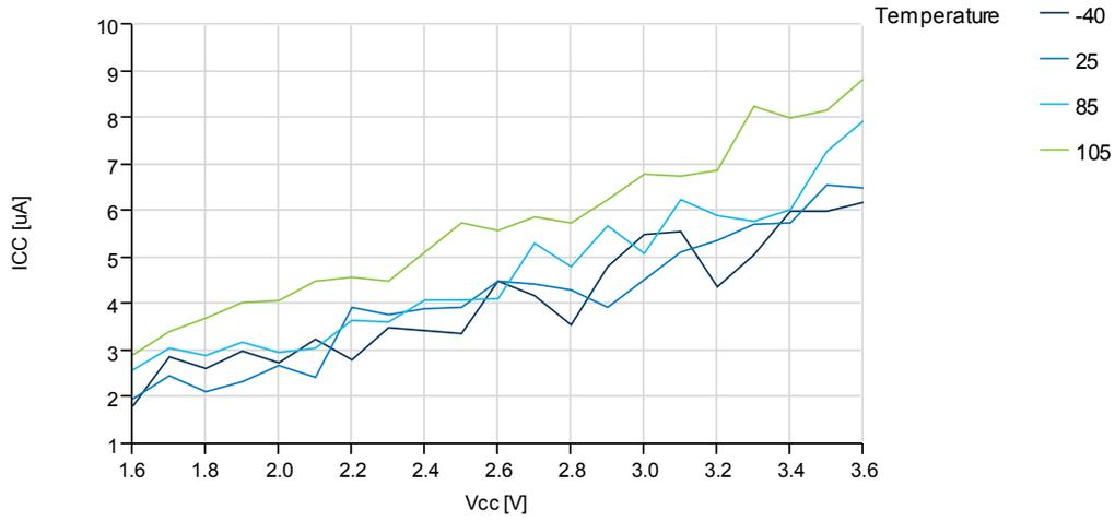
**Figure 37-22. Standby Supply Current vs. V<sub>CC</sub>**
