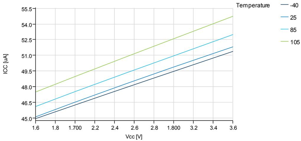
**Figure 37-13. Idle Mode Supply Current vs. V<sub>CC</sub>**
