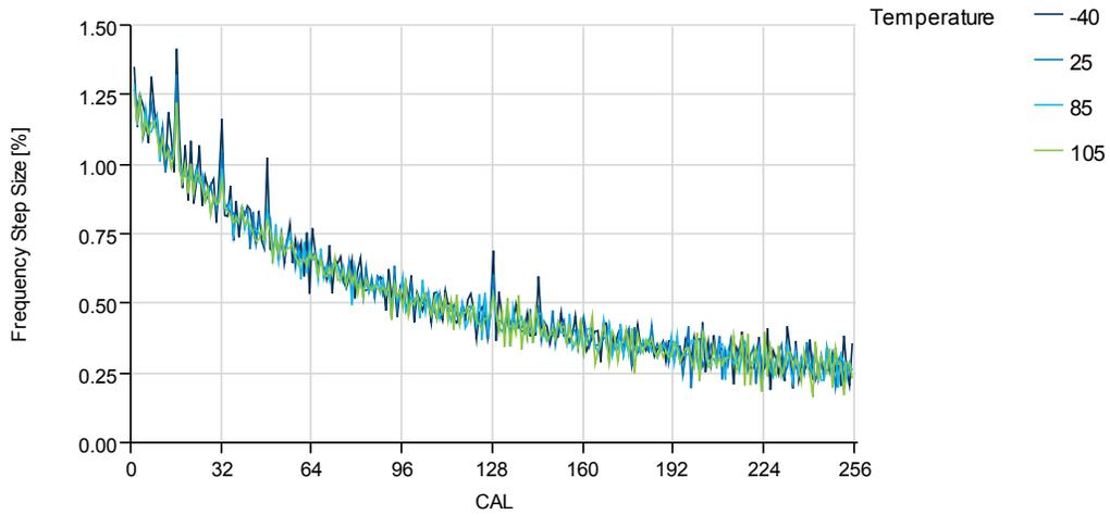
**Figure 37-77. 8MHz Internal Oscillator Frequency vs. Calibration**
