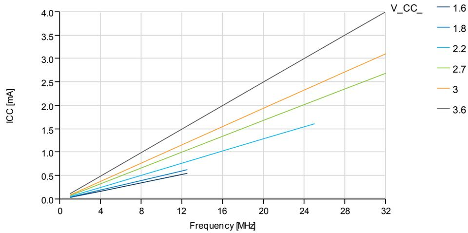
**Figure 37-11. Idle Mode Supply Current vs. V<sub>CC</sub>**
