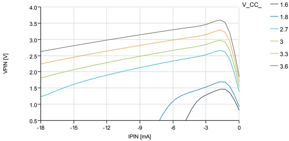
**Figure 37-30. I/O Pin Output Voltage vs. Sink Current**
