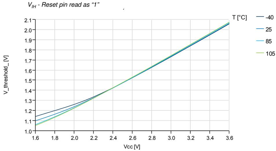
**Figure 37-67. Reset Pin Input Threshold Voltage vs.  $V_{CC}$**
