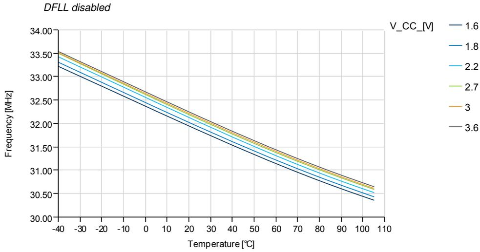
Figure 37-79. 32MHz Internal Oscillator Frequency vs. Temperature
