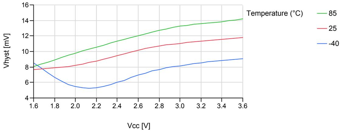
**Figure 37-51. Analog Comparator Hysteresis vs. V<sub>CC</sub>**
