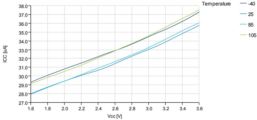
**Figure 37-4. Active Mode Supply Current vs. V<sub>CC</sub>**
