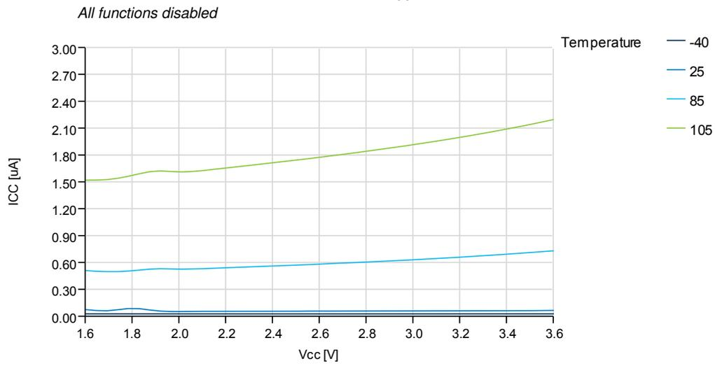
**Figure 37-19. Power-down Mode Supply Current vs. Temperature**
