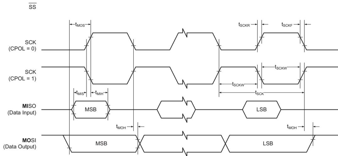
Figure 36-6. SPI Timing Requirements in Slave Mode
