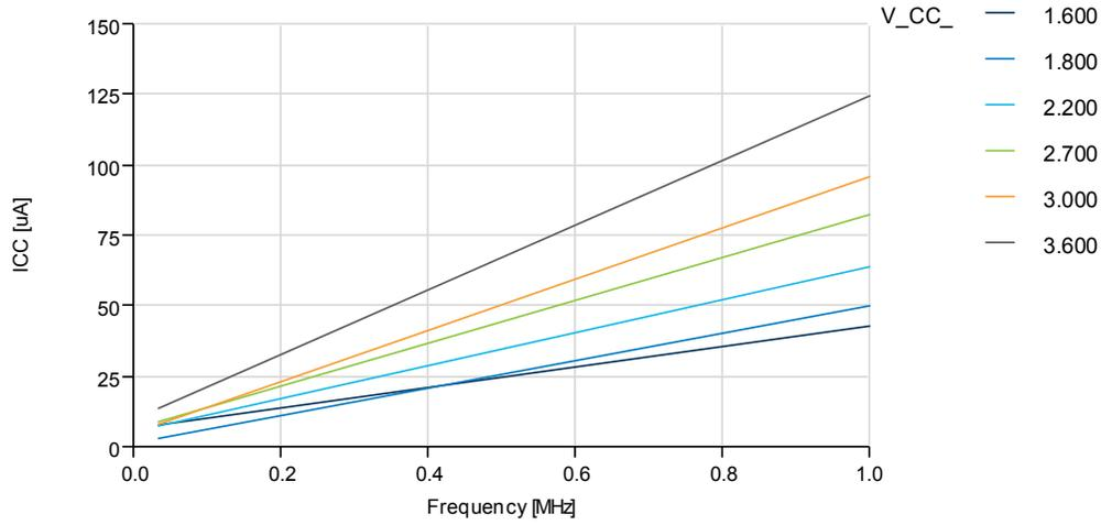
**Figure 37-10. Idle Mode Supply Current vs. Frequency**
