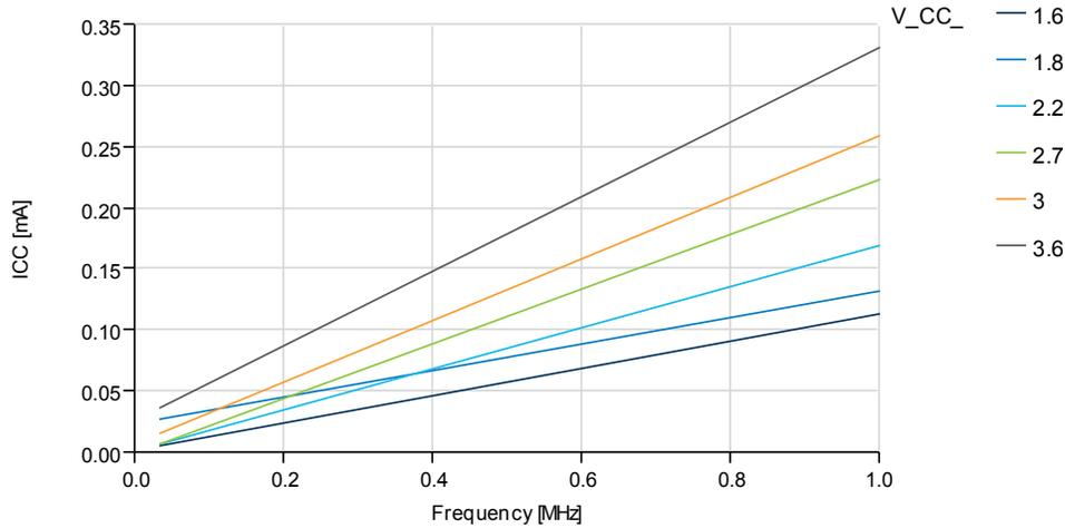
Figure 37-2. Active Mode Supply Current vs. Frequency
