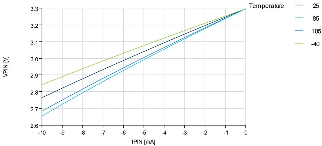
**Figure 37-29. I/O Pin Output Voltage vs. Source Current**
