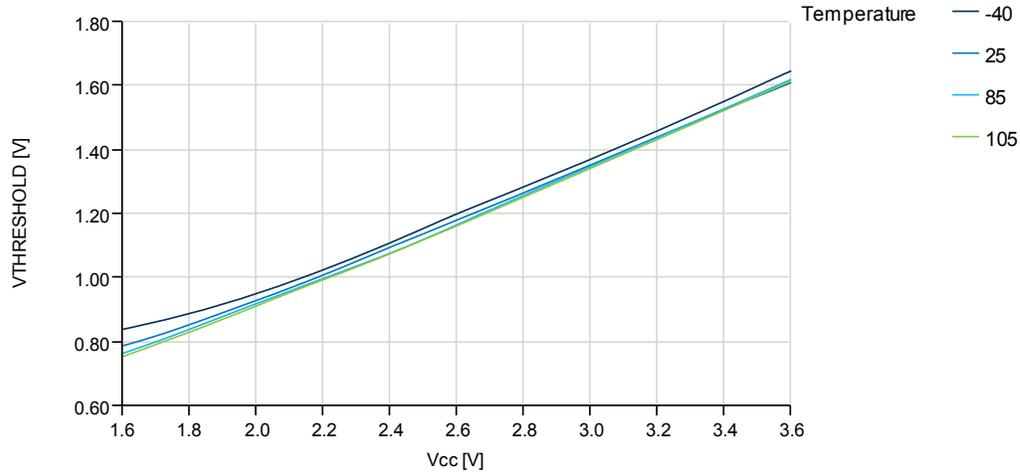
**Figure 37-36. I/O Pin Input Threshold Voltage vs.  $V_{CC}$**
