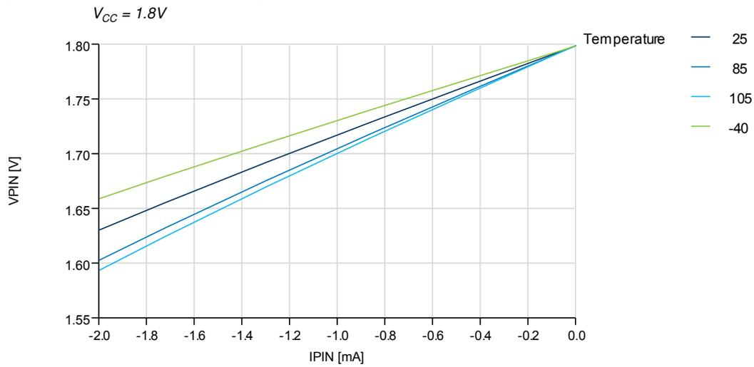
Figure 37-27. I/O Pin Output Voltage vs. Source Current
