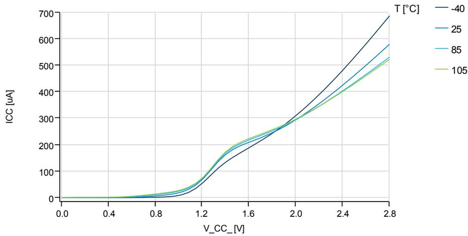
**Figure 37-69. Power-on Reset Current Consumption vs.  $V_{CC}$**
