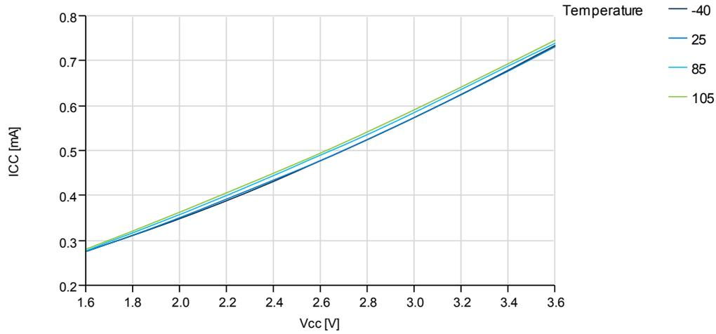
**Figure 37-6. Active Mode Supply Current vs. V<sub>CC</sub>**
