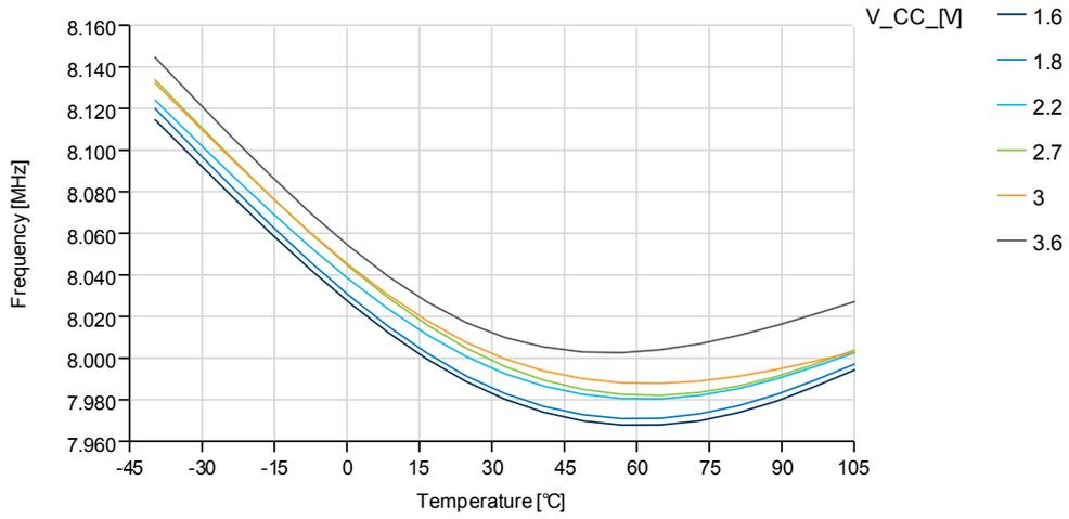
Figure 37-75. 8MHz Internal Oscillator Frequency vs. Temperature
