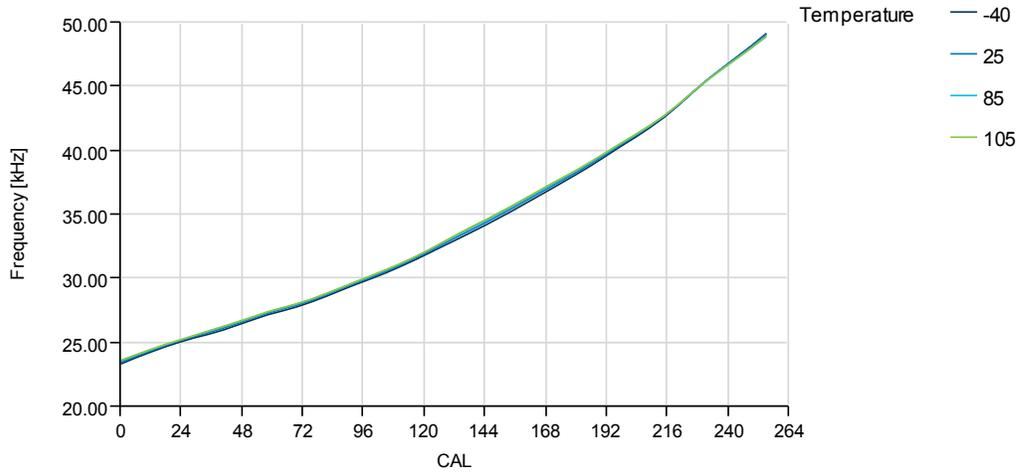
**Figure 37-73. 32.768kHz Internal Oscillator Calibration Step Size**
