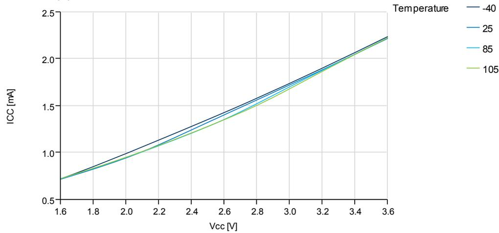
**Figure 37-7. Active mode Supply Current vs. V<sub>CC</sub>**
