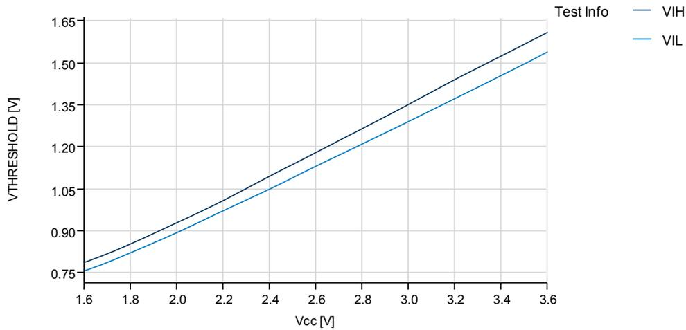
**Figure 37-35. I/O Pin Input Threshold Voltage vs.  $V_{CC}$**
