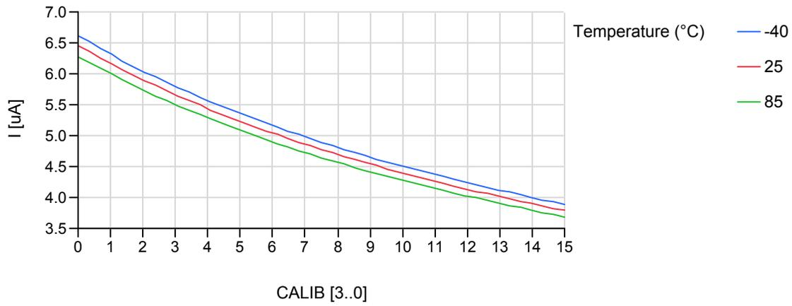
**Figure 37-58. Analog Comparator Source vs. Calibration Value**
