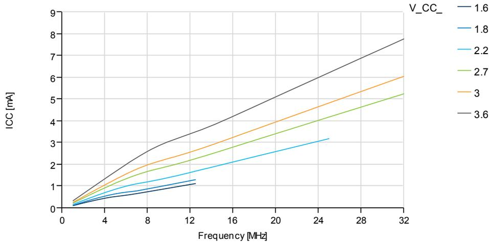
**Figure 37-3. Active Mode Supply Current vs. V<sub>CC</sub>**
