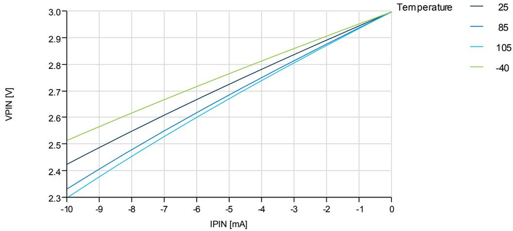
Figure 37-28. I/O Pin Output Voltage vs. Source Current
