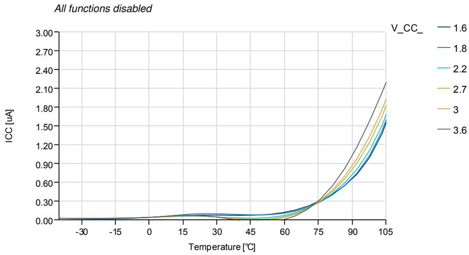
Figure 37-18. Power-down Mode supply Current vs. V<sub>CC</sub>
