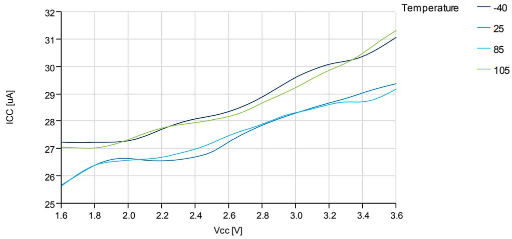
**Figure 37-12. Idle Mode Supply Current vs. V<sub>CC</sub>**
