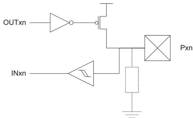
Figure 16-6. I/O Configuration - Wired-AND with Optional Pull-up
