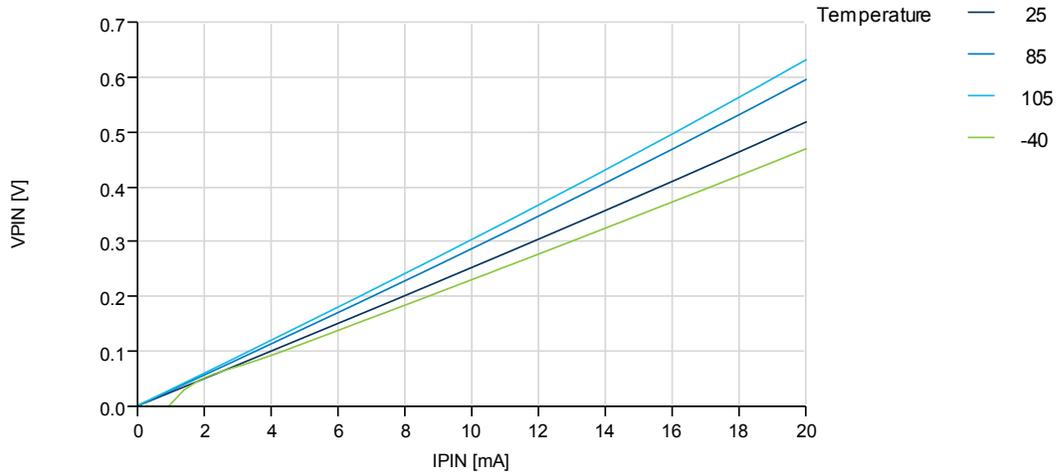
**Figure 37-32. I/O Pin Output Voltage vs. Sink Current**
