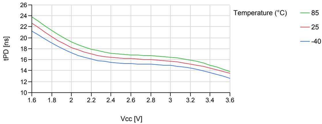
Figure 37-53. Analog Comparator Propagation Delay vs. Temperature
