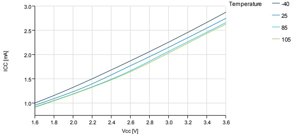
**Figure 37-8. Active Mode Supply Current vs. V<sub>CC</sub>**
