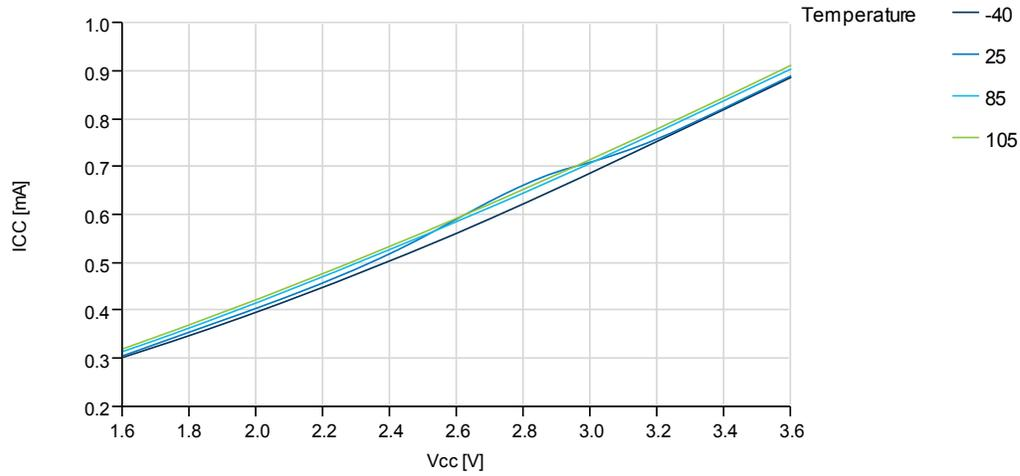
**Figure 37-14. Idle Mode Supply Current vs. V<sub>CC</sub>**
