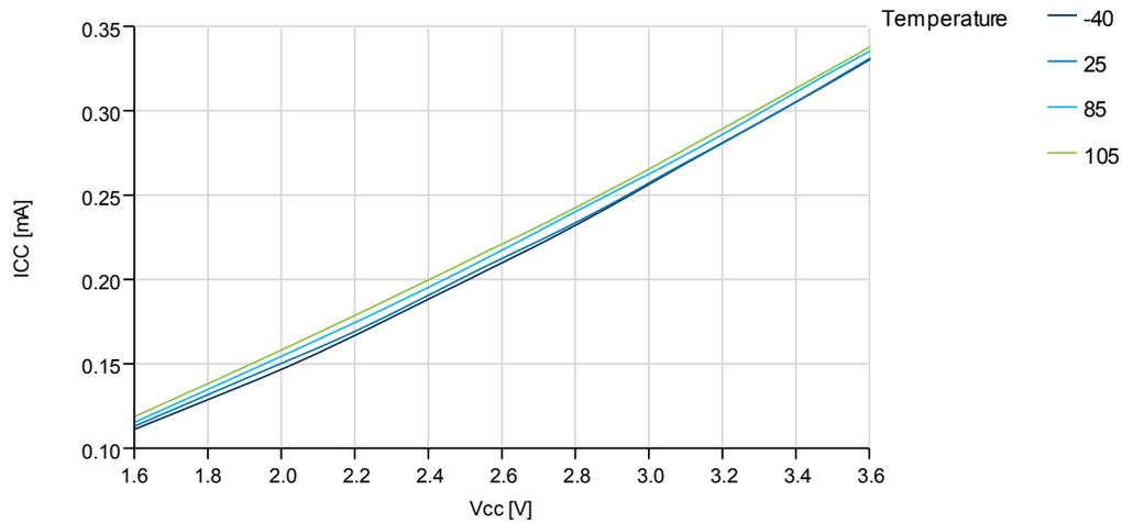
**Figure 37-5. Active Mode Supply Current vs. V<sub>CC</sub>**
