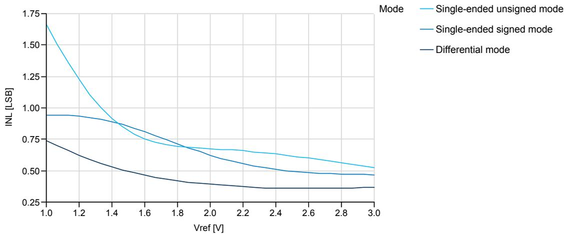
**Figure 37-39. ADC INL Error vs.  $V_{CC}$**
