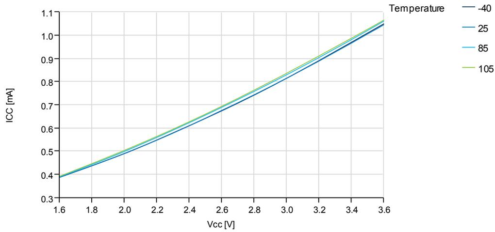
**Figure 37-15. Idle Mode Supply Current vs. V<sub>CC</sub>**
