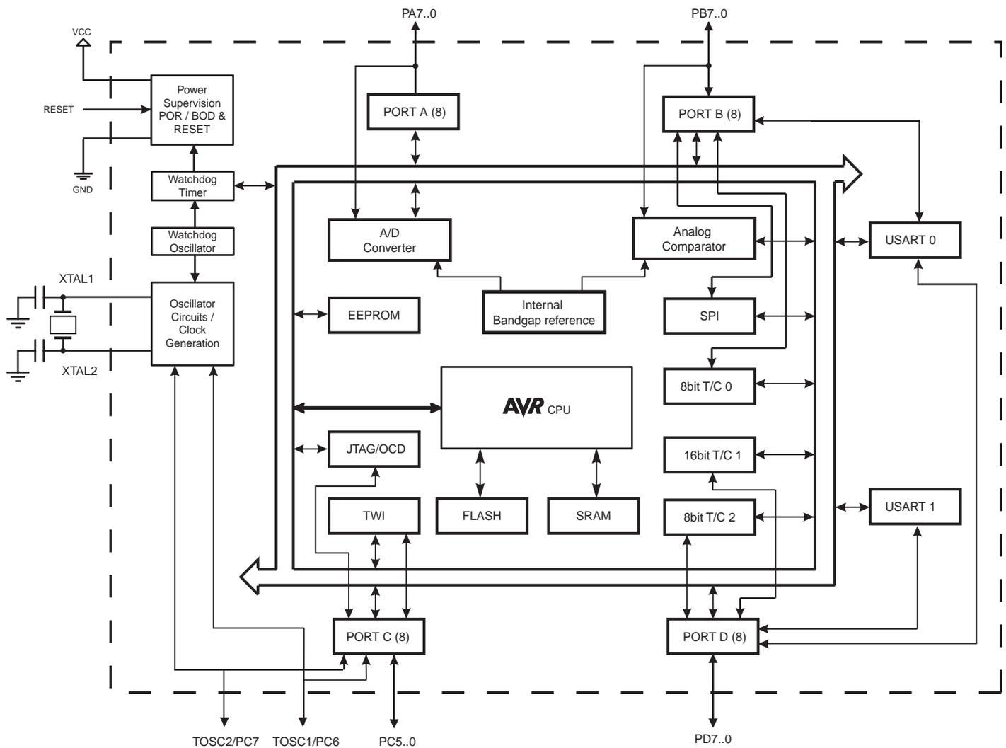
The AVR core combines a rich instruction set with 32 general purpose working registers. All the 32 registers are directly connected to the Arithmetic Logic Unit (ALU), allowing two independent registers to be accessed in one single instruction executed in one clock cycle. The resulting
