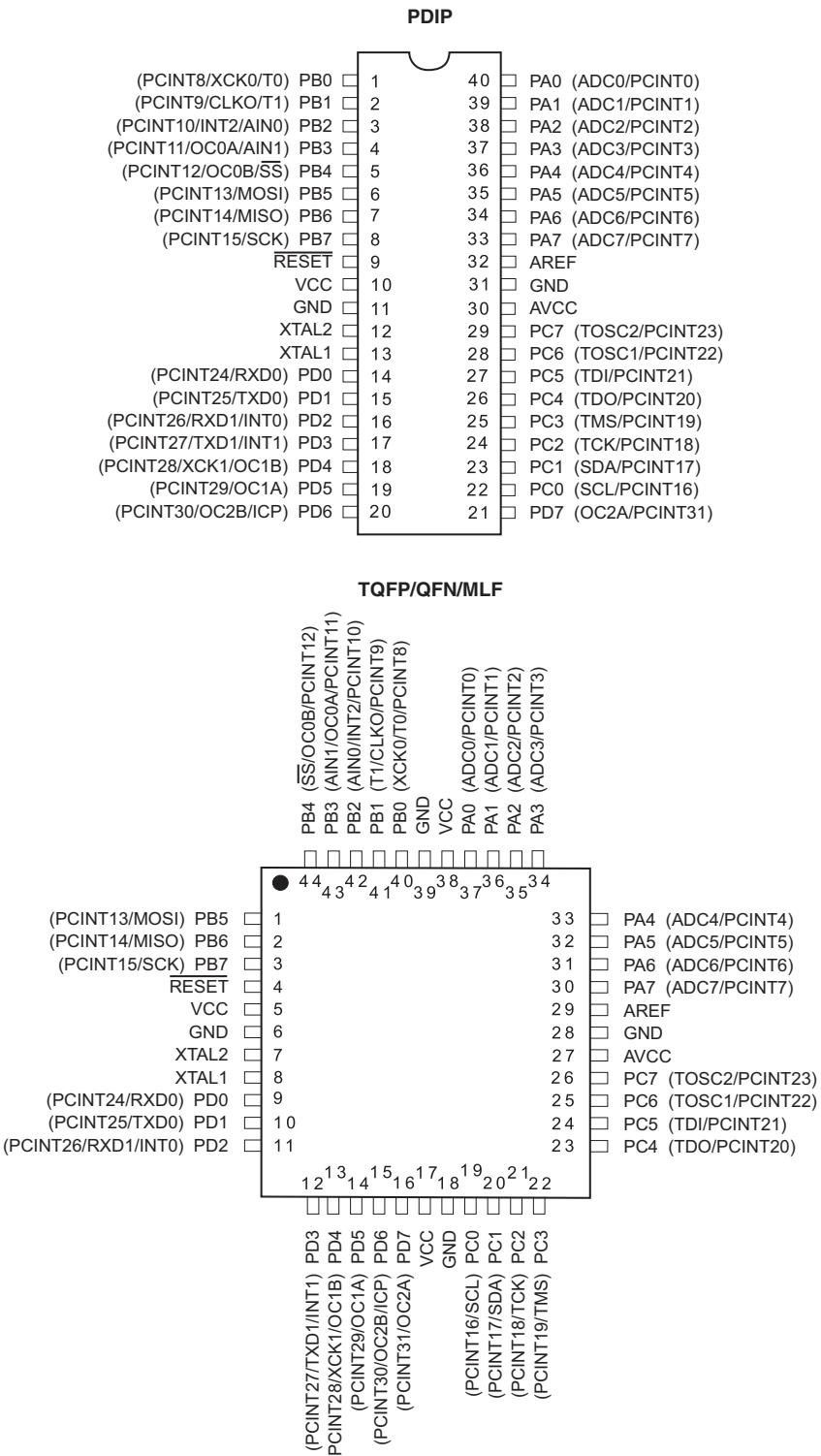
Note: The large center pad underneath the QFN/MLF package should be soldered to ground on the board to ensure good mechanical stability.
