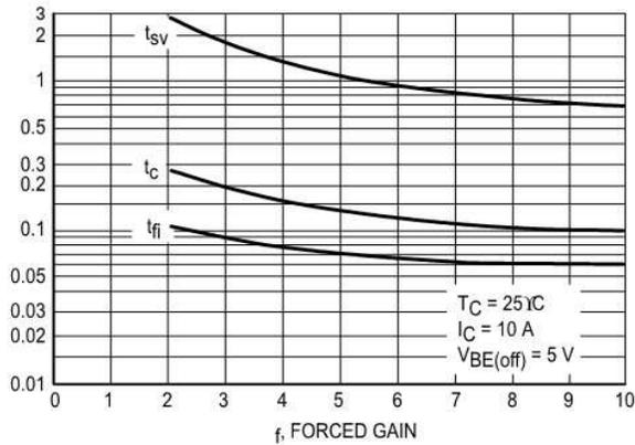
**Figure 11a. Turn-Off Times versus Forced Gain**
