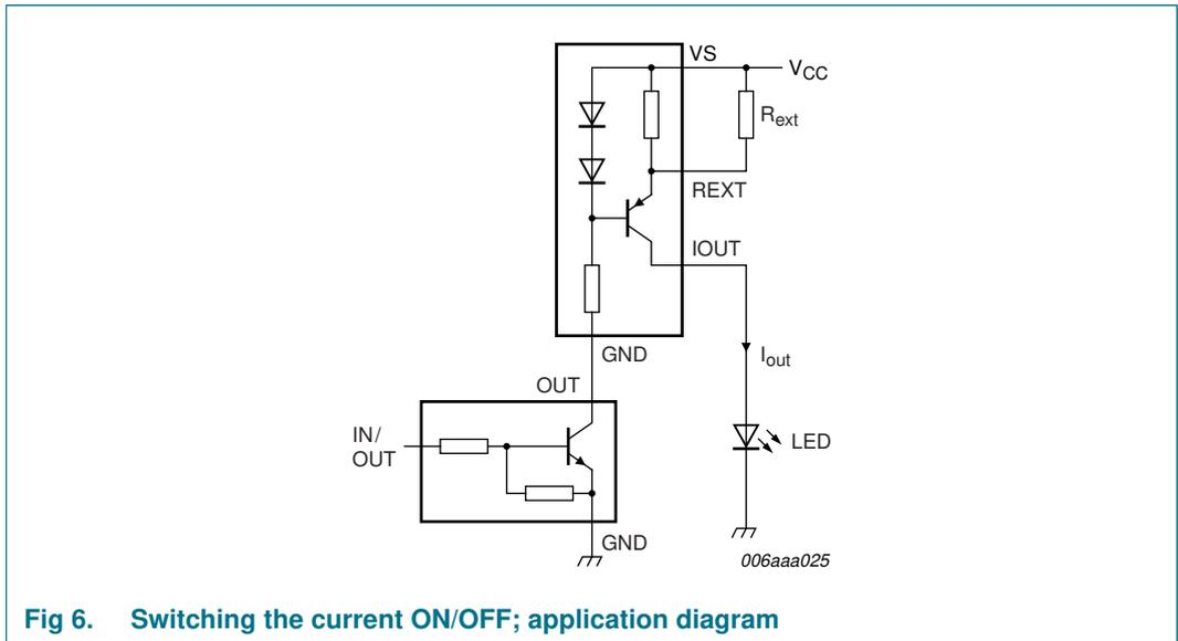
Fig 6. Switching the current ON/OFF; application diagram
