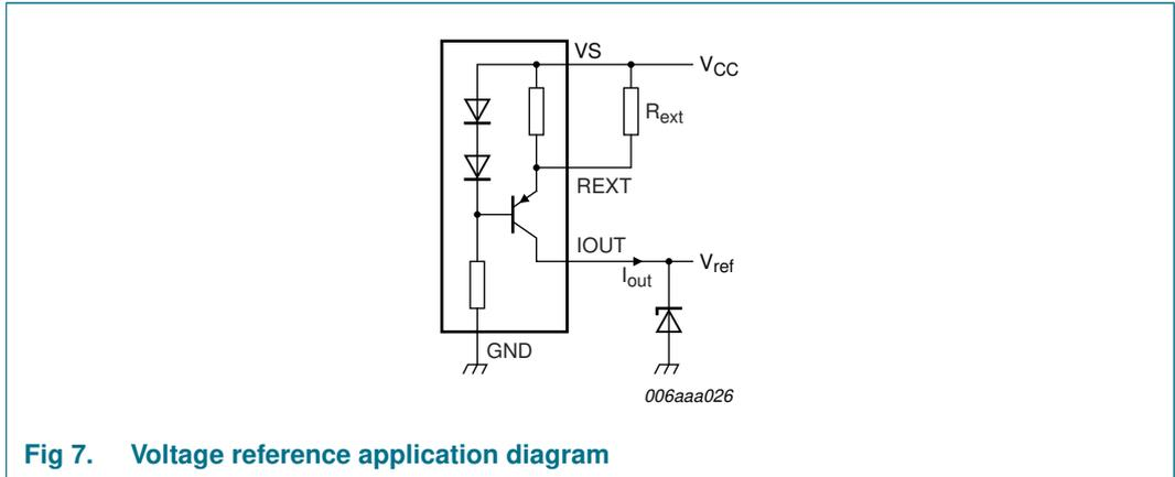
**Fig 7. Voltage reference application diagram**
