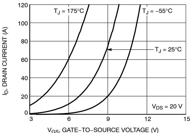
Figure 5. Transfer Characteristics
