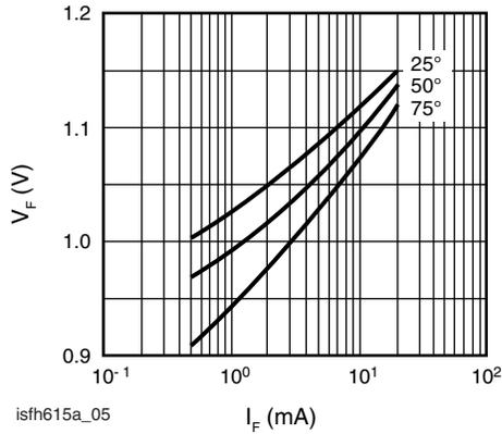
Fig. 6 - Diode Forward Voltage (typ.) vs. Forward Current
