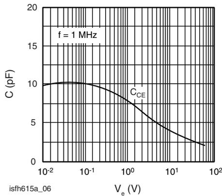
Fig. 7 - Transistor Capacitance (typ.) vs. Collector Emitter Voltage
