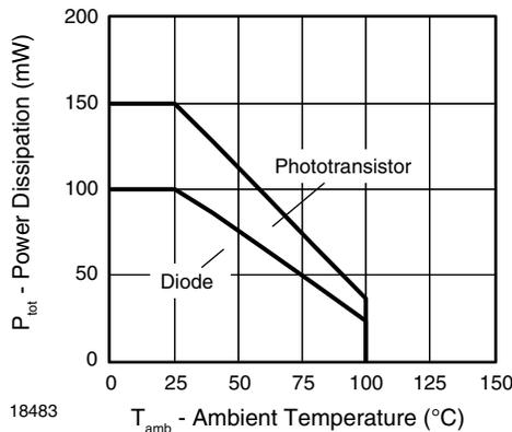
Fig. 1 - Permissible Power Dissipation vs. Ambient Temperature
