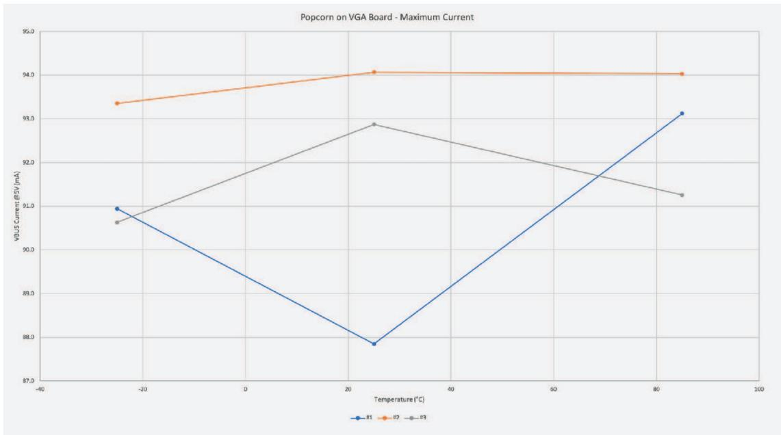
Table 2. Popcorn running on the VGA Board (VGA video, SD Card and I2S audio) with power saving disabled (GPI023 pulled high)
