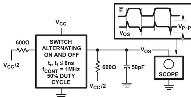
Figure 13. Control to Switch Feedthrough Noise Test Circuit
