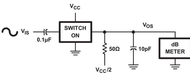
Figure 10. Frequency Response Test Circuit
