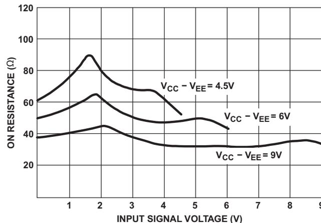
**Figure 21. Typical ON Resistance vs Input Signal Voltage**
