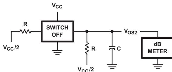
Figure 11. Crosstalk Between Two Switches Test Circuit
