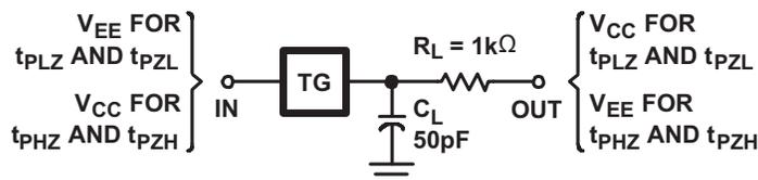
Figure 15. Switch ON/OFF Propagation Delay Test Circuit
