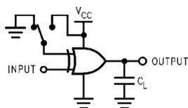
C<sub>L</sub> includes load and stray capacitance
