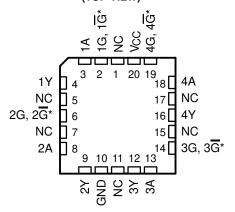
\*\$\overline{G}\$ on '125 and 'LS125A devices; G on 126 and 'LS126A devices NC - No internal connection
