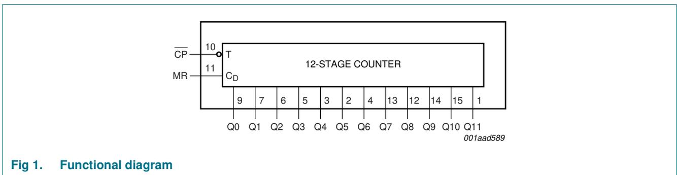
**Fig 1. Functional diagram**
