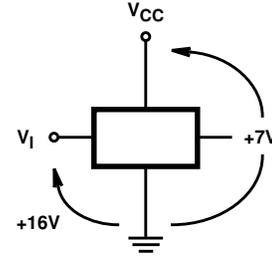
**CAUTION:** Stresses above those listed in "Absolute Maximum Ratings" may cause permanent damage to the device. This is a stress only rating and operation of the device at these or any other conditions above those indicated in the operational sections of this specification is not implied.
