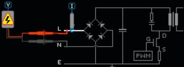
Current harmonics analysis measures the amplitude of frequency components that can be injected back into the AC lines. Therefore, FFT analysis with flat top window is performed. Current harmonics analysis also performs pre-compliance testing according to standards EN 61000-3-2 A / B / C / D.
