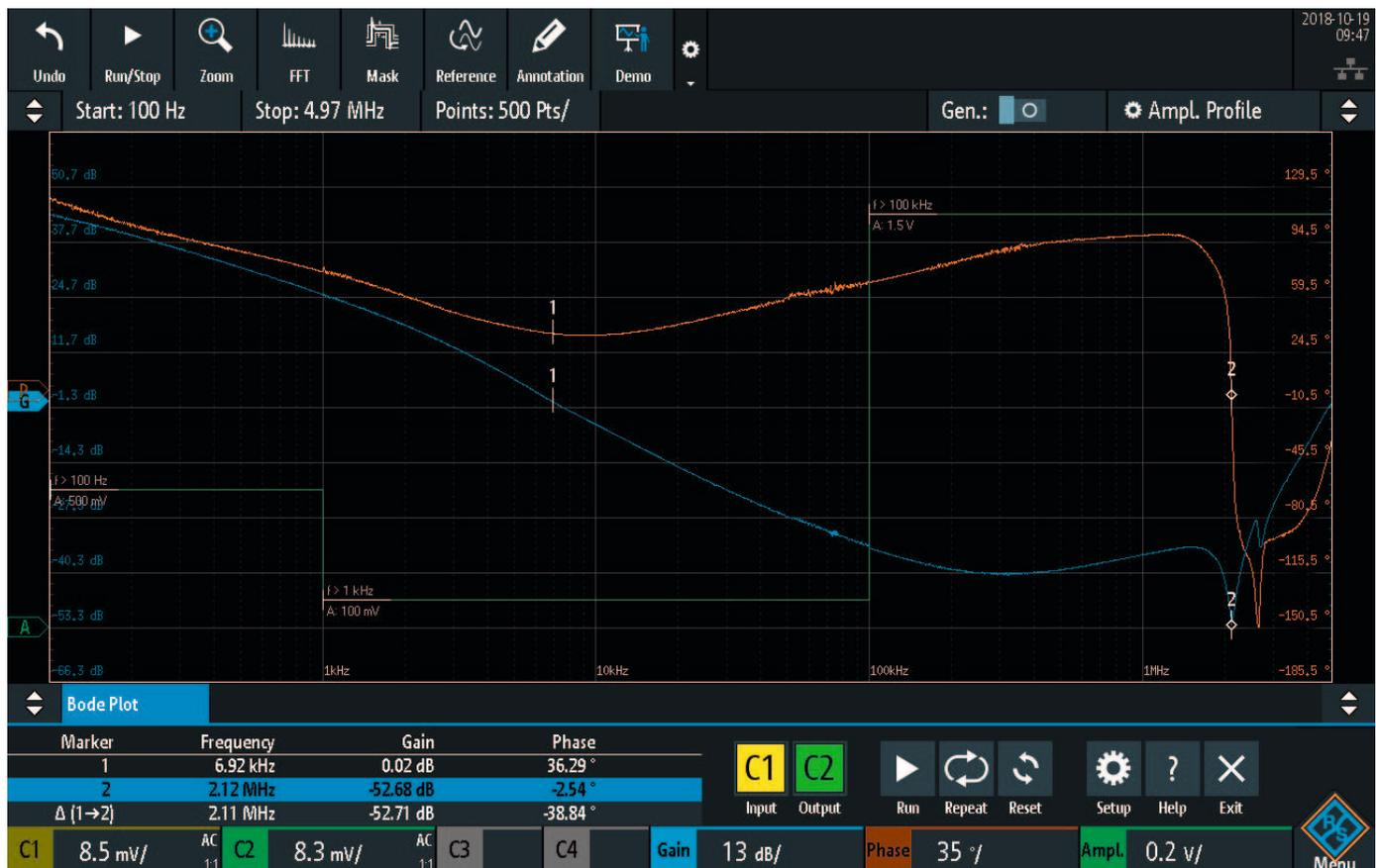
The R&S®RTM-K36 frequency response analysis (Bode plot) option characterizes the frequency response of a variety of electronic devices, including passive filters and amplifier circuits
