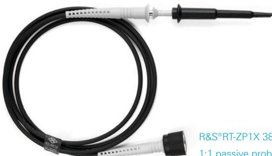
R&S®RT-ZP1X 38 MHz bandwidth 1:1 passive probe
