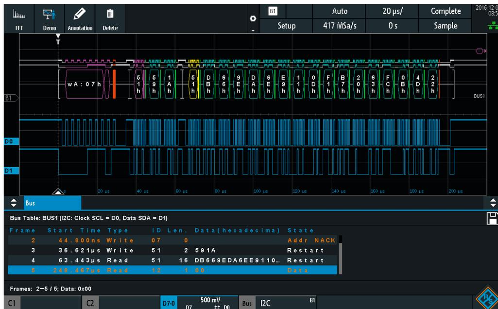
Decoded hexadecimal I<sup>2</sup>C message shown in honeycomb format and in table
