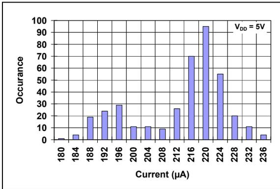
**FIGURE 2-12:**  $I_{DD}$  Histogram .
