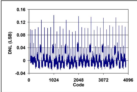
**FIGURE 2-1:** DNL vs. Code ( $V_{DD} = 5.5\text{V}$ ).
