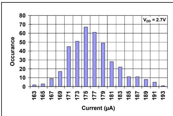
**FIGURE 2-13:**  $I_{DD}$  Histogram.
