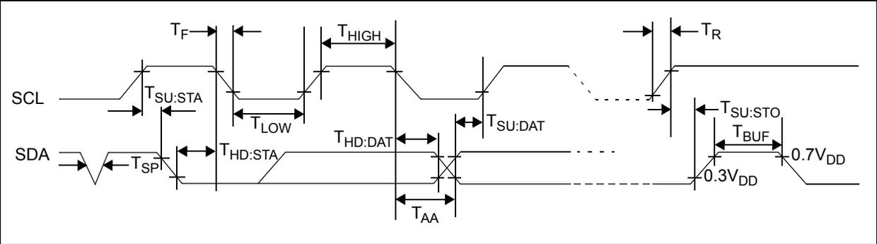
FIGURE 7-4: I<sup>2</sup>C Bus Timing Data.
