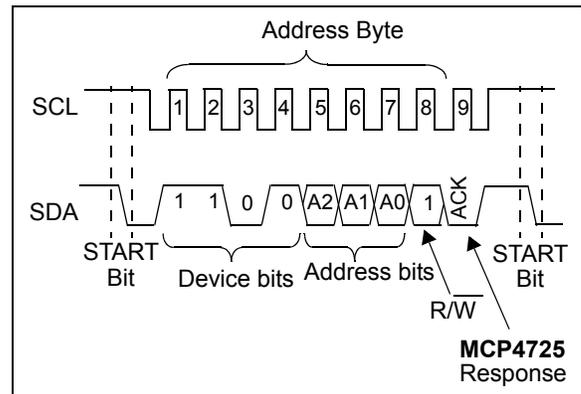
**FIGURE 8-2:** I<sup>2</sup>C Bus Connection Test.
