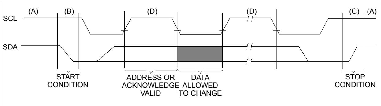
**FIGURE 7-3:** Data Transfer Sequence On The Serial Bus.
