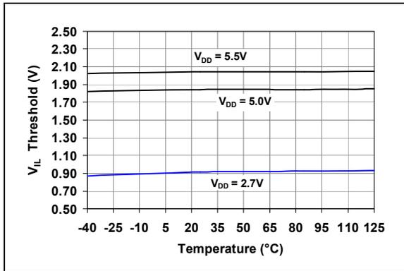
**FIGURE 2-18:**  $V_{IL}$  Low Threshold vs. Temperature and  $V_{DD}$ .
