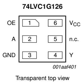
Fig 6. Pin configuration SOT891, SOT1115 and SOT1202
