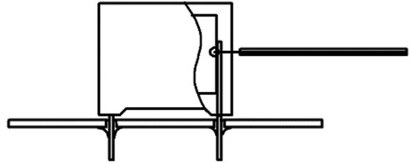
*Temperature monitored inside the capacitor.*
