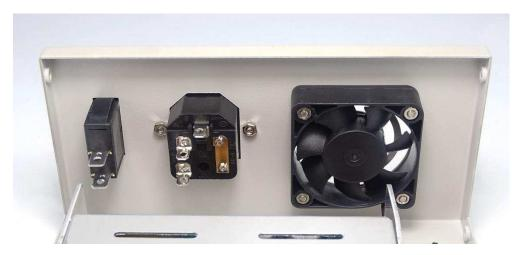
4 Install the switch power supply: install the switch power supply on the lower board.
