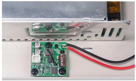
8 Install RD6006: install RD6006 on the front side and connect the external sensor.
