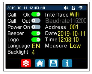
Turn on the "Call out", the output will be turn on automatically when you call out a data group. If you turn it off, the output will keep the previous status.
