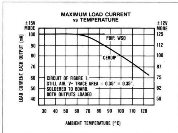
Figure 2. Maximum Load Current Vs. Temperature
