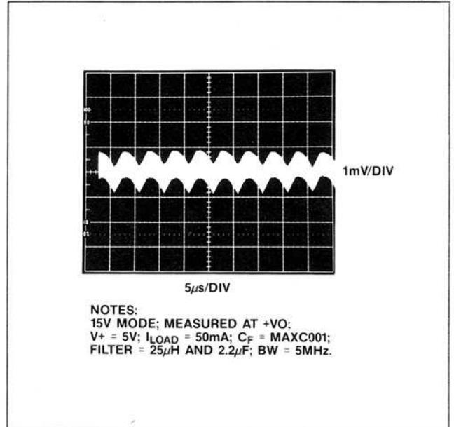
Figure 9. Output Noise Voltage with Pi Filter
