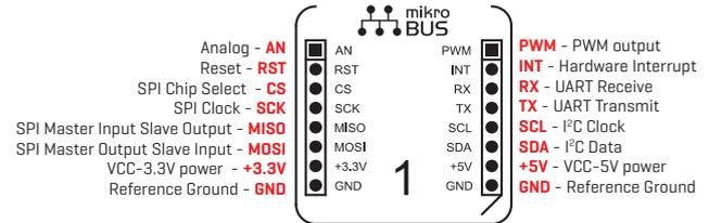
click boards™ are made in accordance with mikroBUS™ — a standard that defines their size, shape, 16-pin connector and corresponding mainboard socket. It is an open standard. Independent developers can implement mikroBUS™ sockets on their own boards to take full advantage of click boards™.
