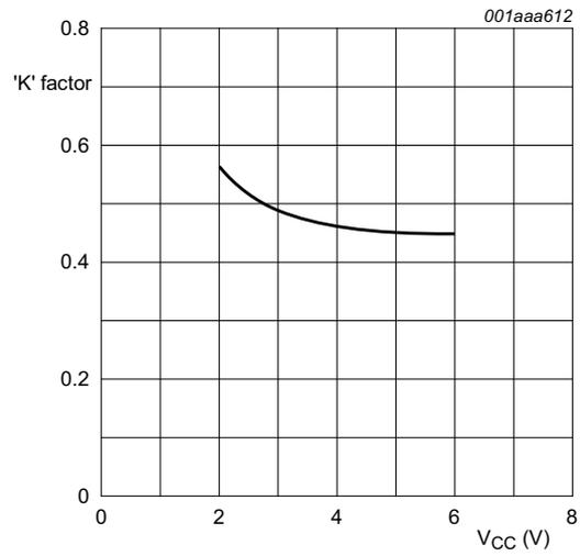
$C_{EXT} = 10\text{ nF}; R_{EXT} = 10\text{ k}\Omega\text{ to }100\text{ k}\Omega.$
