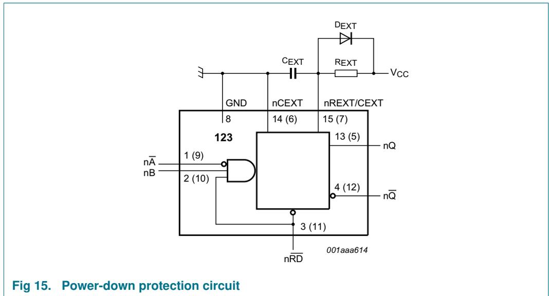
Fig 15. Power-down protection circuit
