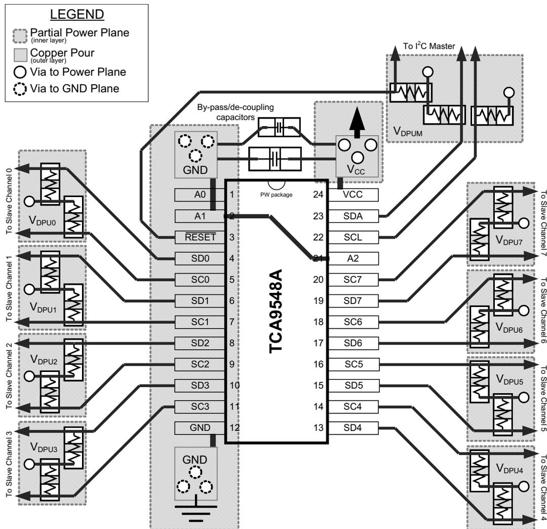
Figure 20. Layout Schematic
