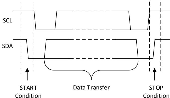
**Figure 7. Definition of Start and Stop Conditions**
