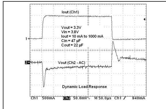
**FIGURE 2-29:** Dynamic Load Response (10 mA to 1000 mA).
