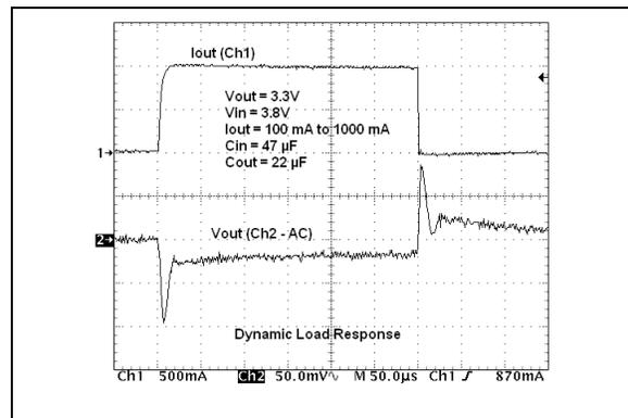
**FIGURE 2-30:** Dynamic Load Response (100 mA to 1000 mA).
