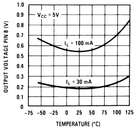
Figure 7-10. Typical Output Voltage vs Temperature
