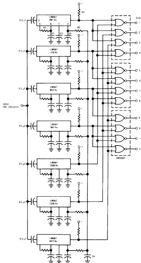
Component values (typ) R1 6.8 to 15k R2 4.7k R3 20k C1 0.10 mfd C2 1.0 mfd 6V C3 2.2 mfd 6V C4 250 mfd 6V
