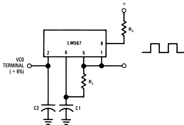
Figure 10-7. Precision Oscillator Drive 100-mA Loads
