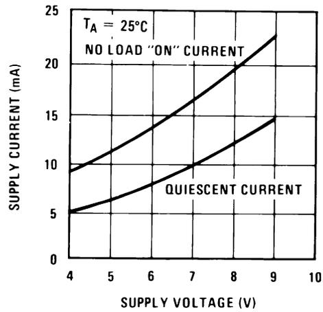
Figure 7-8. Typical Supply Current vs Supply Voltage
