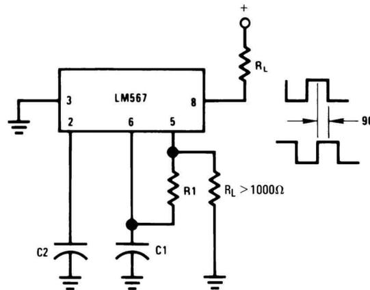
Connect Pin 3 to 2.8V to Invert Output
