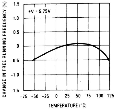
Figure 7-1. Typical Frequency Drift
