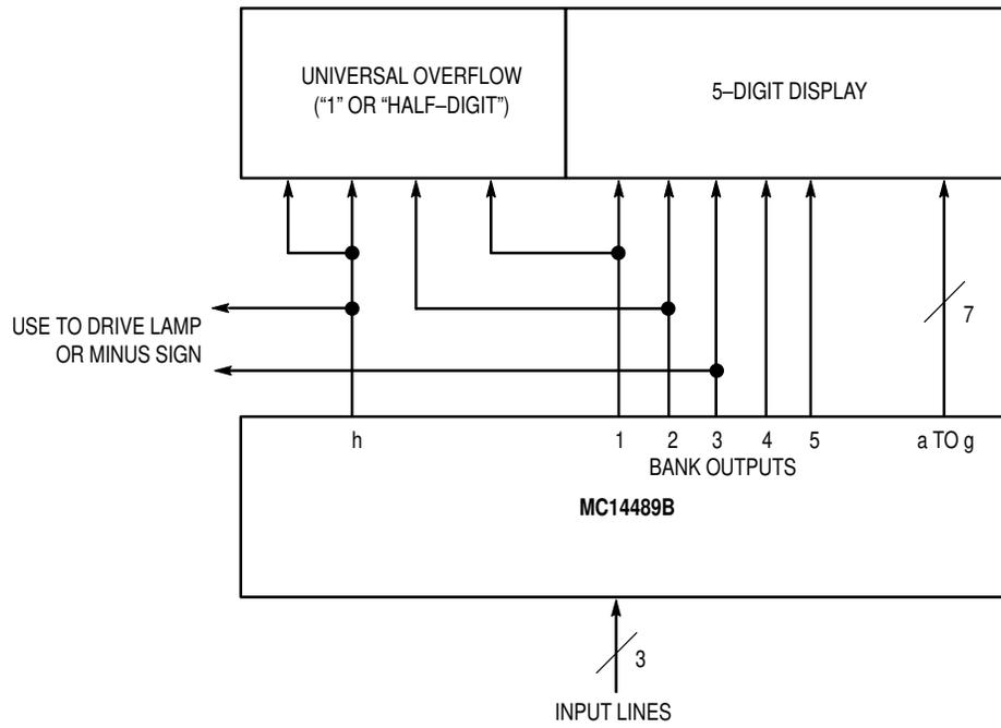
NOTE: A Universal Overflow pins out all anodes and cathodes.
