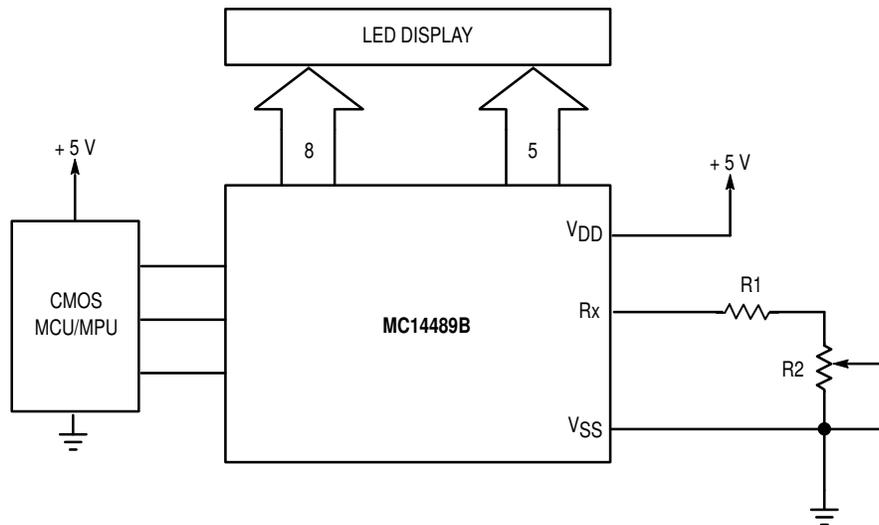
NOTE: R1 limits the maximum current to avoid damaging the display and/or the MC14489B due to overheating. See the Thermal Considerations section. An 1/8 watt resistor may be used for R1. R2 is a 1 kΩ or 5 kΩ potentiometer ( $\geq 1/8$  watt). R2 may be a light-sensitive resistor.
