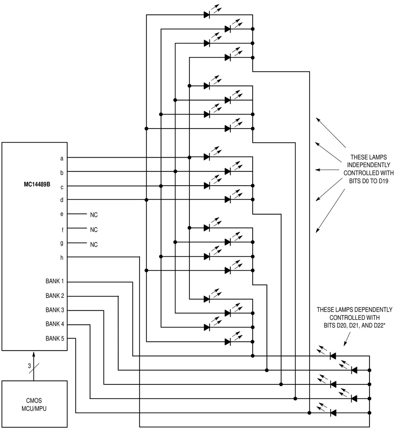
\* If required, this group of lamps can be independently controlled. To accomplish independent control, only connect lamps to BANK 1 and BANK 2 for output h (two lamps). Then, use bits D20, D21, and D22 for control of these two lamps.
