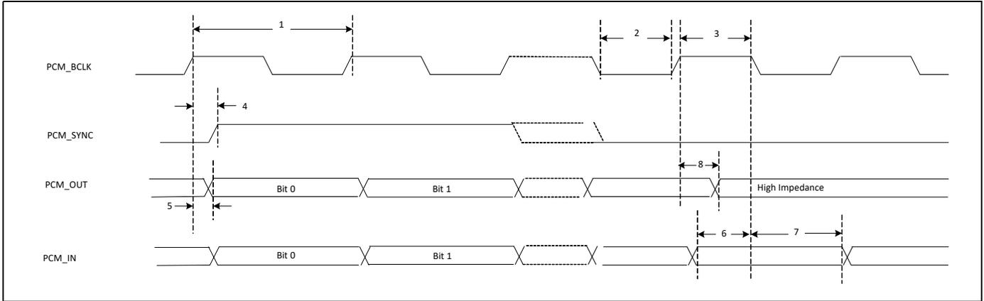
Table 10. PCM Interface Timing Specifications (Long Frame Sync, Master Mode)
