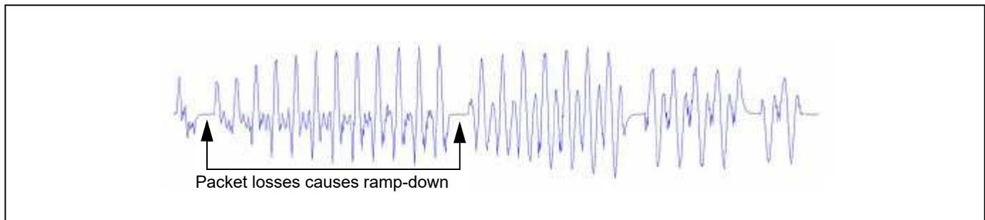
Figure 19. CVSD Decoder Output Waveform After Applying PLC
