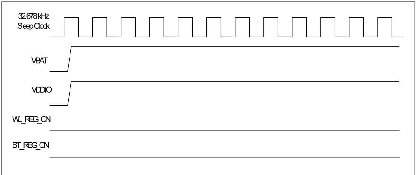
Figure 34. WLAN = ON, Bluetooth = OFF
