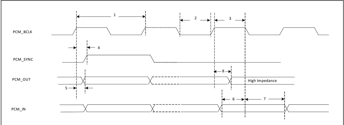
Table 8. PCM Interface Timing Specifications (Short Frame Sync, Master Mode)
