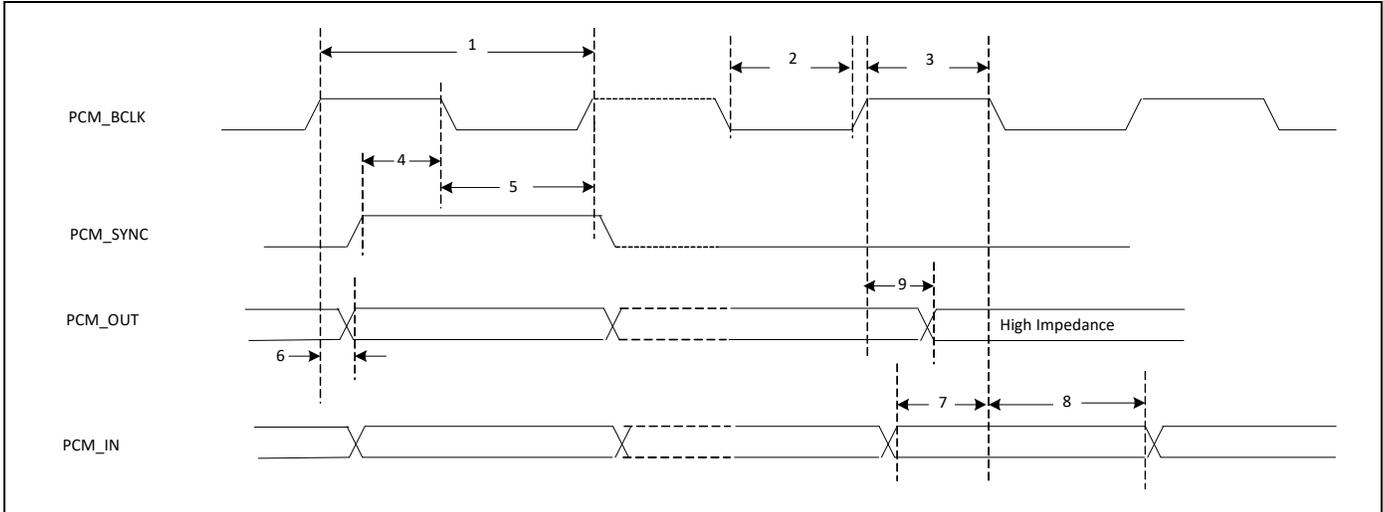
Table 9. PCM Interface Timing Specifications (Short Frame Sync, Slave Mode)
