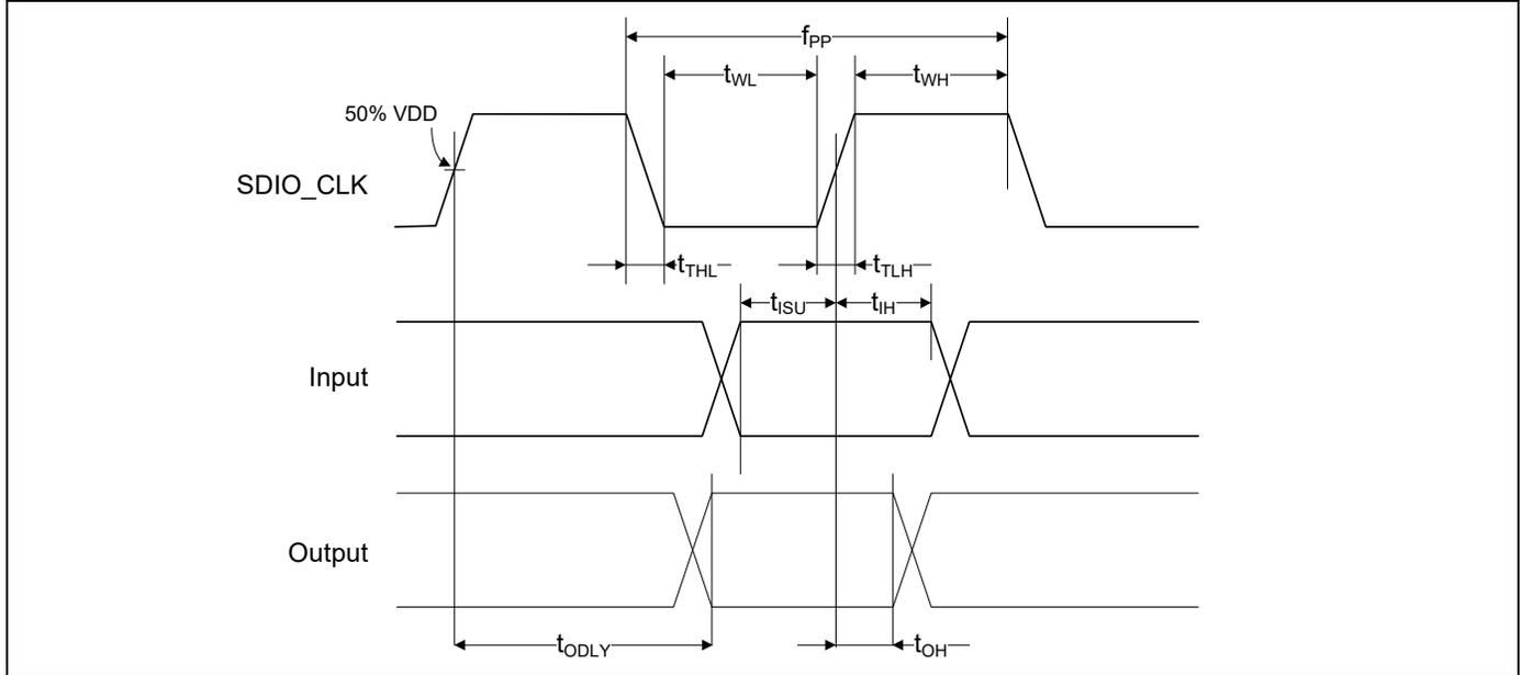
Table 41. SDIO Bus Timing <sup>[56]</sup> Parameters (High-Speed Mode)
