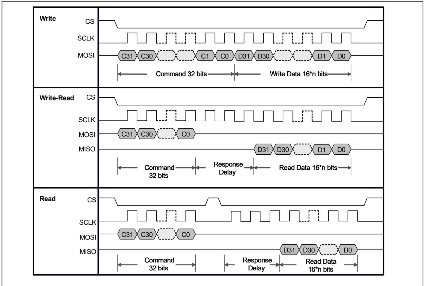
Figure 14. gSPI Signal Timing with Status (Response Delay = 0)
