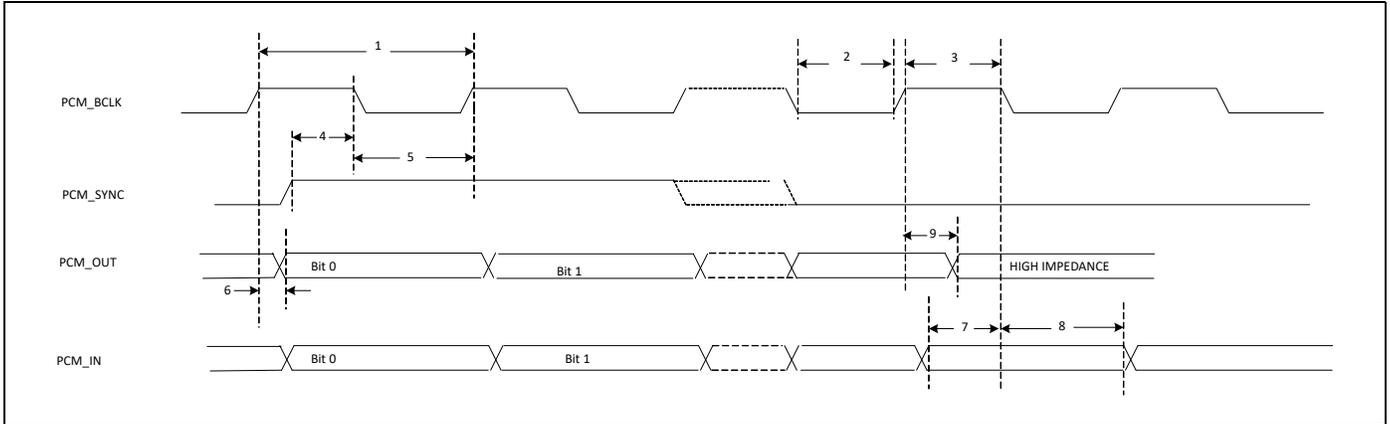
Table 11. PCM Interface Timing Specifications (Long Frame Sync, Slave Mode)
