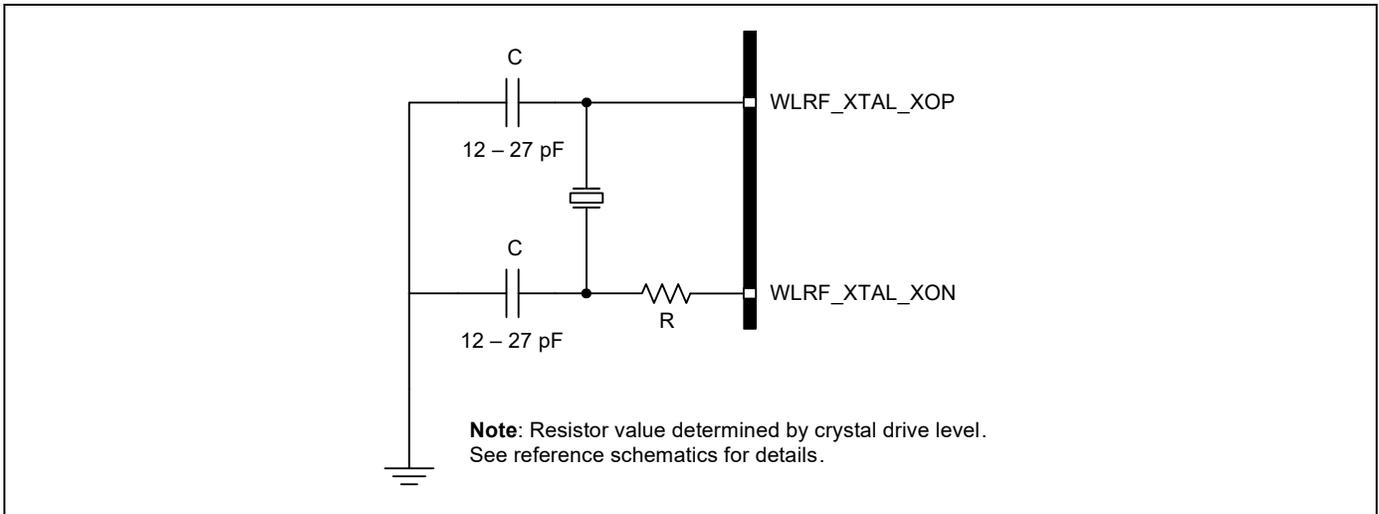
The CYW43439 uses a fractional-N synthesizer to generate the radio frequencies, clocks, and data/packet timing so that it can operate using numerous frequency references. The frequency reference can be an external source such as a TCXO or a crystal interfaced directly to the CYW43439.
