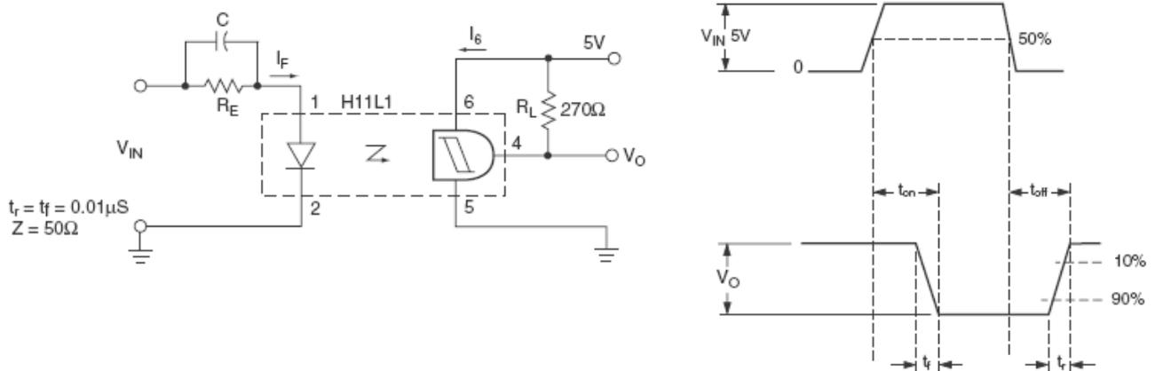
Figure 7. Switching Time Test Circuit & Waveforms
