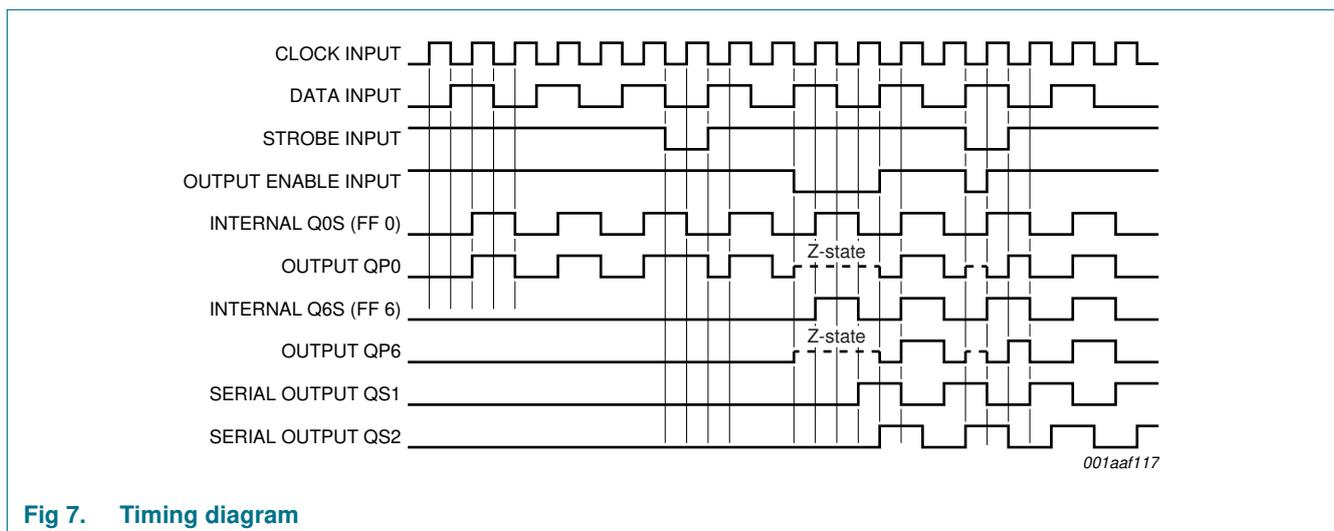
Fig 7. Timing diagram
