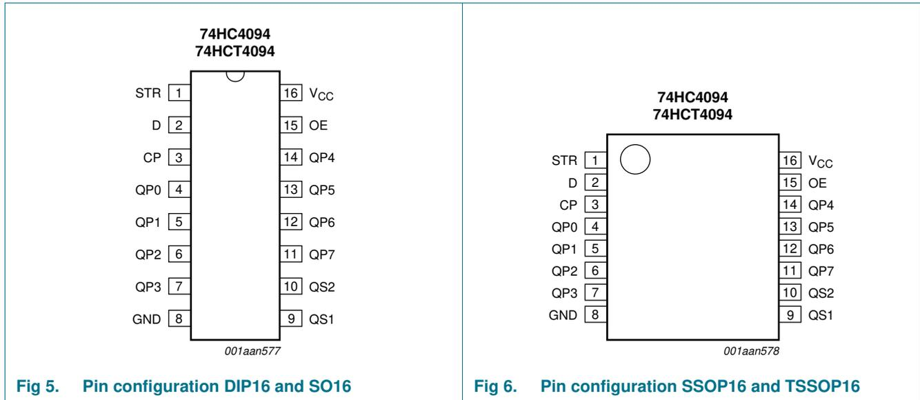
Fig 5. Pin configuration DIP16 and SO16
