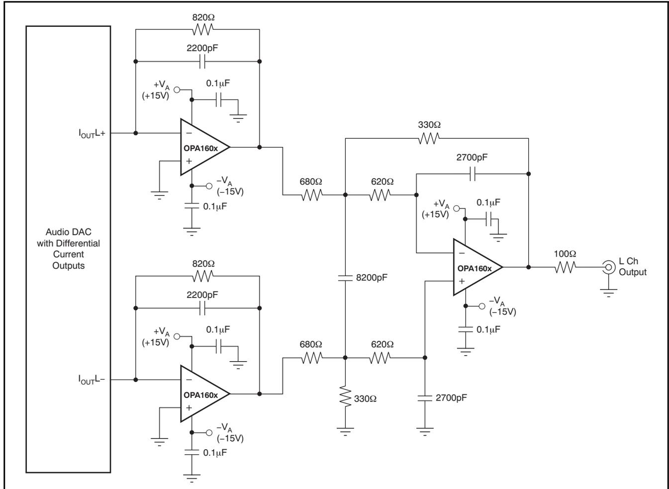
**Figure 37. Audio DAC I/V Converter and Output Filter**
