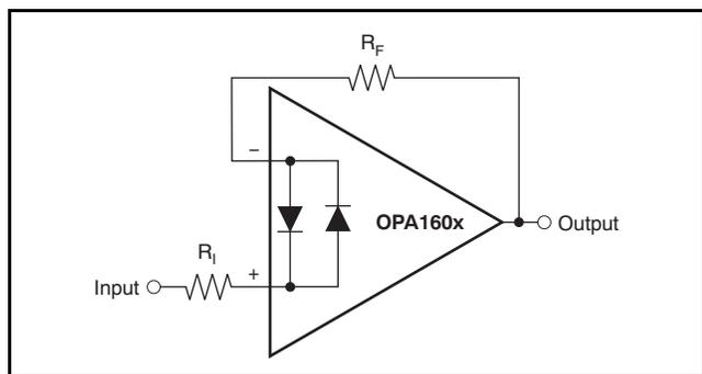
Figure 32. Pulsed Operation
