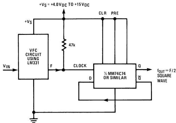
Figure 26. Voltage-to-Frequency Converter with Square-Wave Output Using ÷ 2 Flip-Flop
