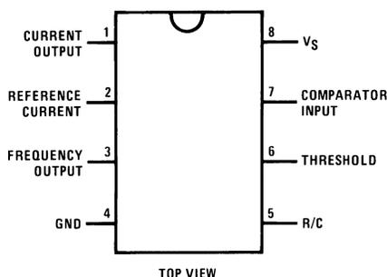
**Figure 1. Plastic Dual-In-Line Package (PDIP)**
