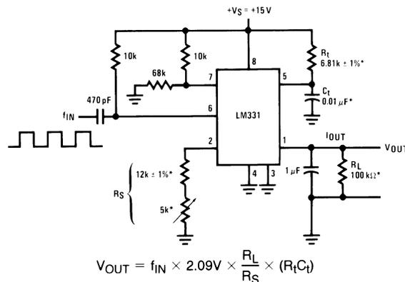
\*Use stable components with low temperature coefficients.
