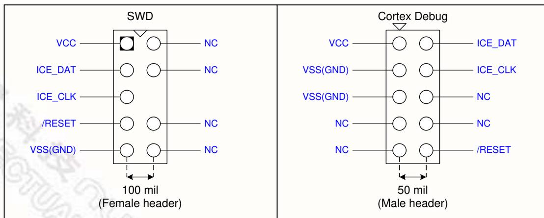
Figure 4-2 SWD and Cortex Debug Connector Pin Diagrams
