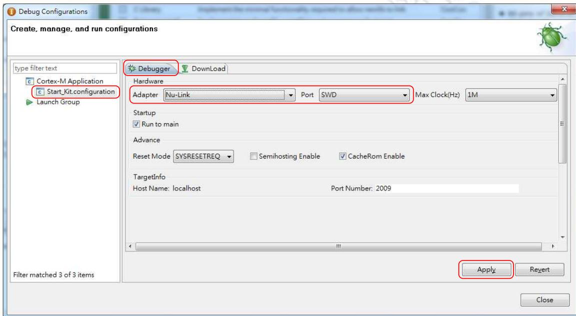
Figure 4-20 Specify the Debugger Options for CooCox CoIDE
