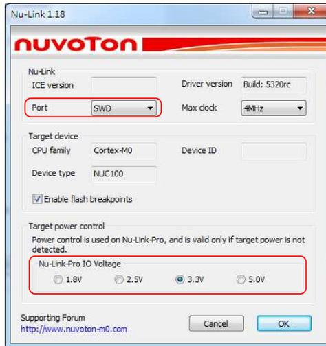
Figure 4-19 Specify the Port and Target I/O Voltage
