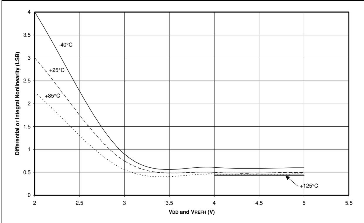
FIGURE 18-24: A/D NONLINEARITY vs. VREFH (VDD = 5V, -40°C TO +125°C)
