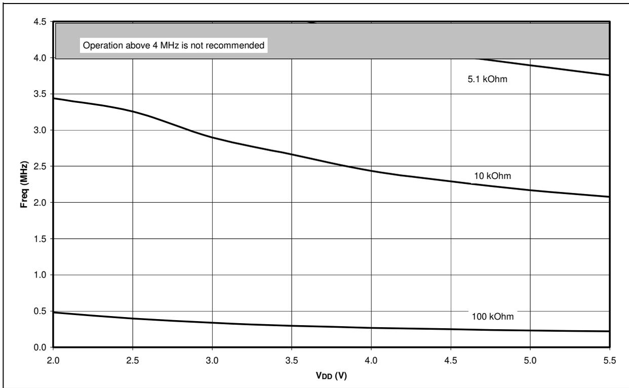
**FIGURE 18-8: AVERAGE  $F_{osc}$  vs.  $V_{DD}$  FOR VARIOUS VALUES OF R (RC MODE,  $C = 100\text{ pF}$ ,  $+25^\circ\text{C}$ )**
