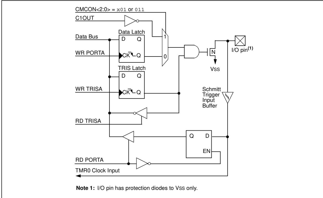
**FIGURE 4-3: BLOCK DIAGRAM OF RA5 PIN**
