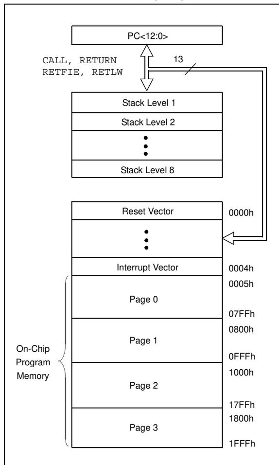
**FIGURE 2-2: PIC16F873A/874A PROGRAM MEMORY MAP AND STACK**
