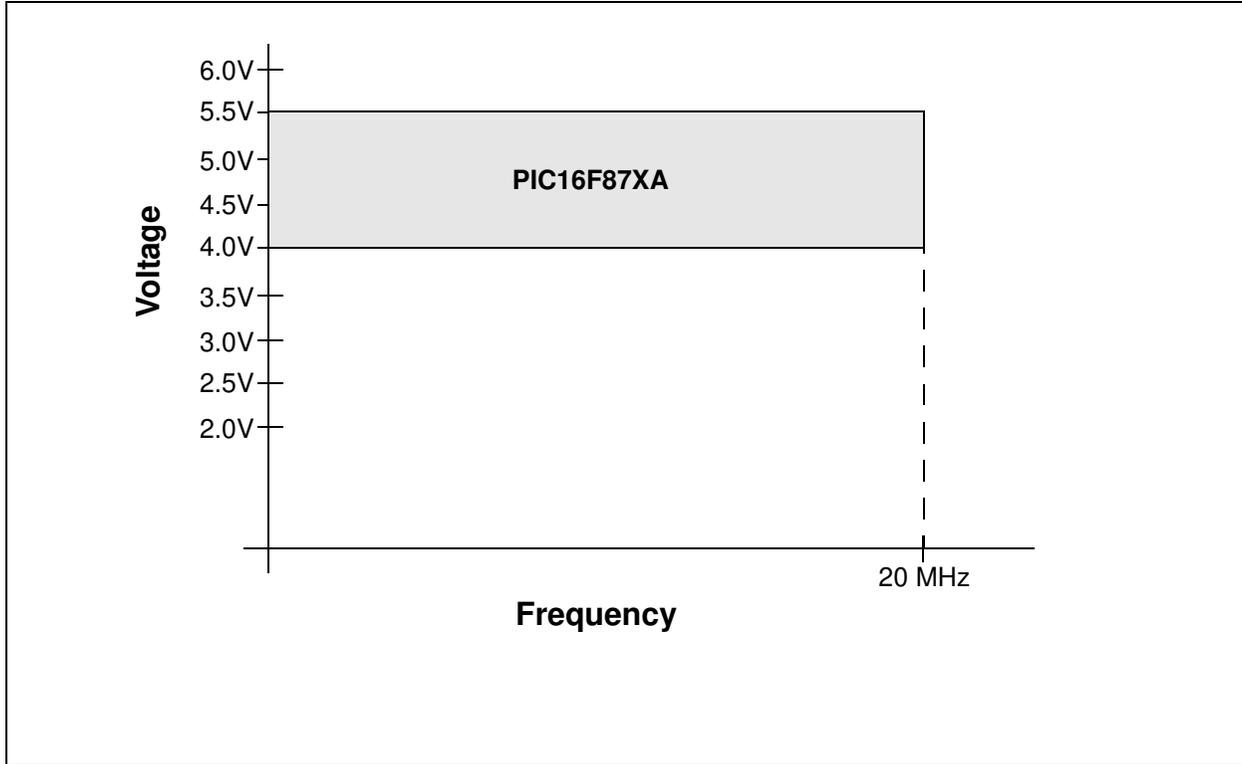
FIGURE 17-2: PIC16LF87XA VOLTAGE-FREQUENCY GRAPH (INDUSTRIAL)
