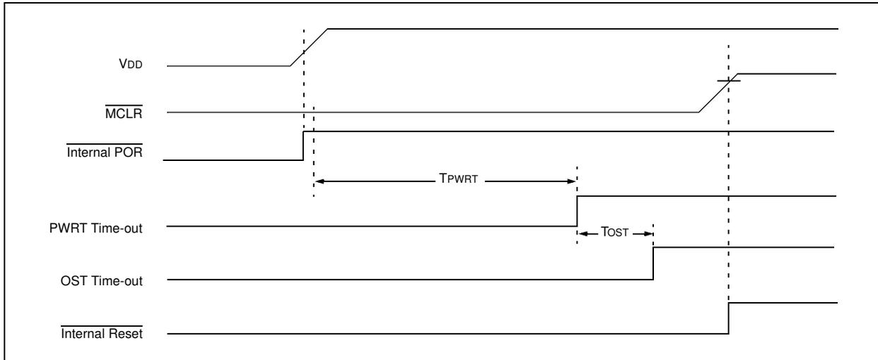
**FIGURE 14-9: SLOW RISE TIME ( $\overline{\text{MCLR}}$  TIED TO  $V_{\text{DD}}$  VIA RC NETWORK)**
