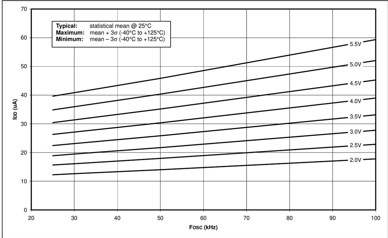
**FIGURE 18-6: MAXIMUM  $I_{DD}$  vs.  $F_{osc}$  OVER  $V_{DD}$  (LP MODE)**
