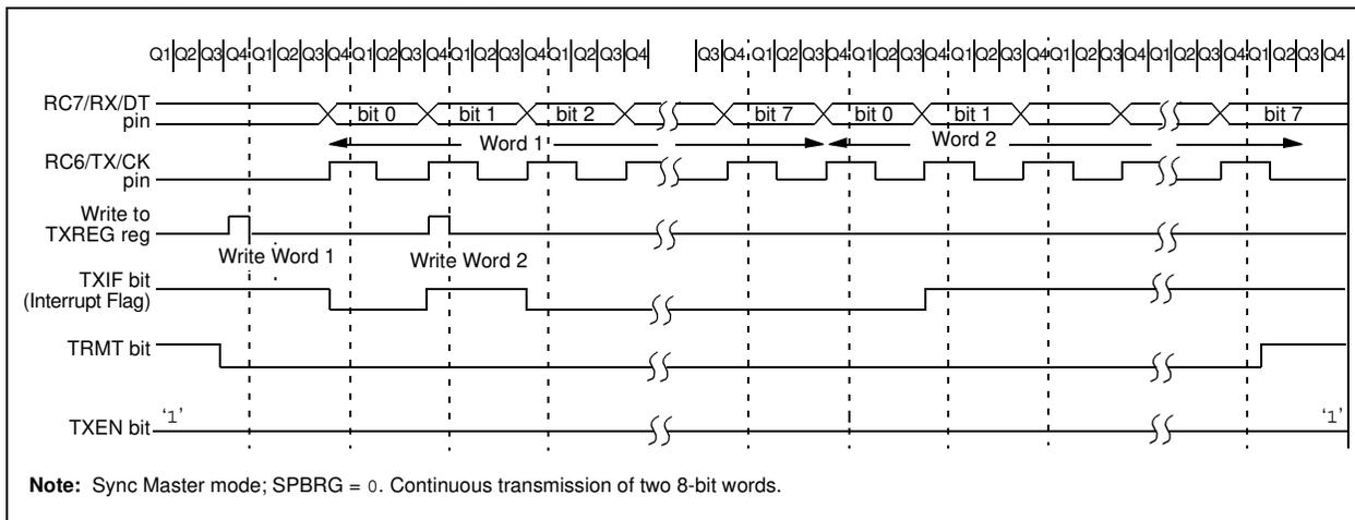
**FIGURE 10-10: SYNCHRONOUS TRANSMISSION (THROUGH TXEN)**
