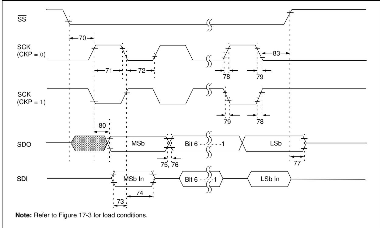
**FIGURE 17-14: SPI SLAVE MODE TIMING (CKE = 1)**
