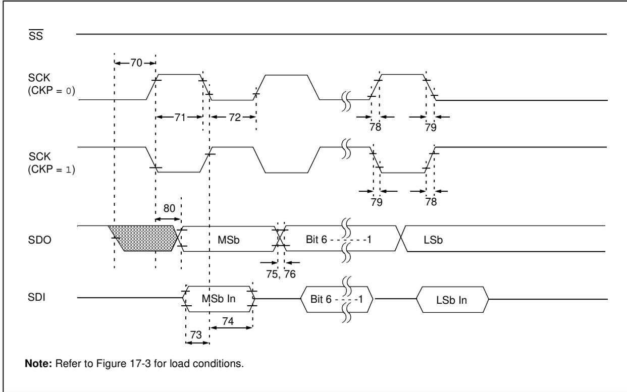
**FIGURE 17-12: SPI MASTER MODE TIMING (CKE = 1, SMP = 1)**
