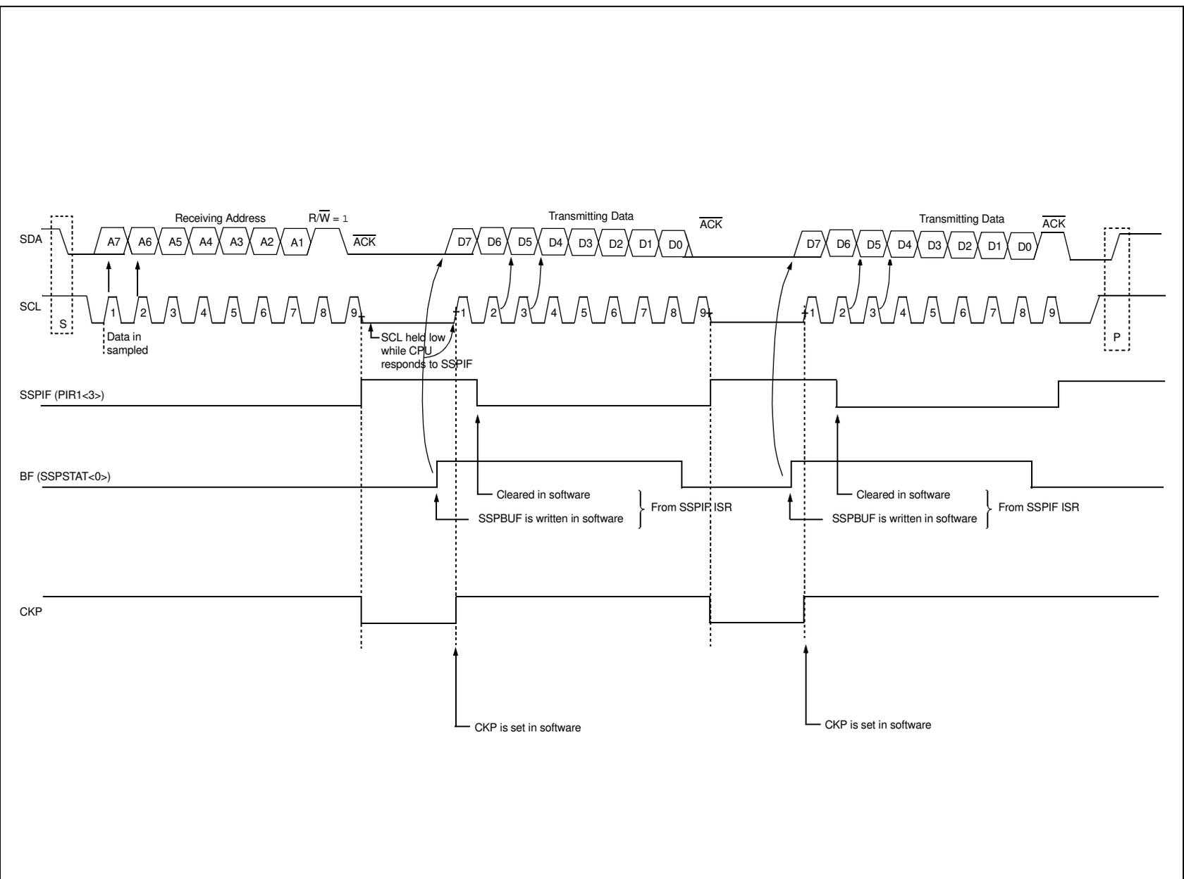
FIGURE 9-10: I<sup>2</sup>C SLAVE MODE TIMING WITH SEN = 0 (RECEPTION, 10-BIT ADDRESS)
