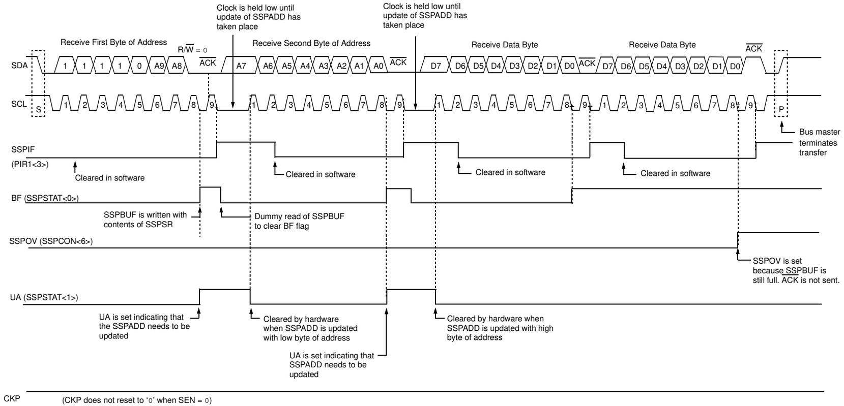
FIGURE 9-11: I<sup>2</sup>C SLAVE MODE TIMING (TRANSMISSION, 10-BIT ADDRESS)
