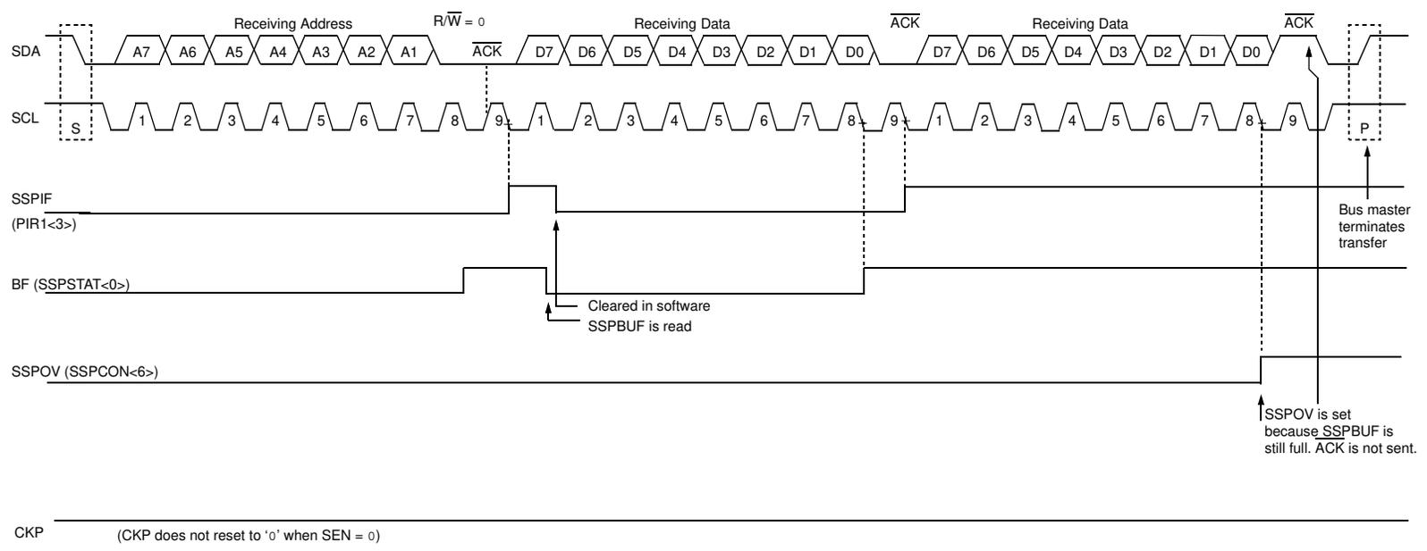
FIGURE 9-9: I<sup>2</sup>C SLAVE MODE TIMING (TRANSMISSION, 7-BIT ADDRESS)
