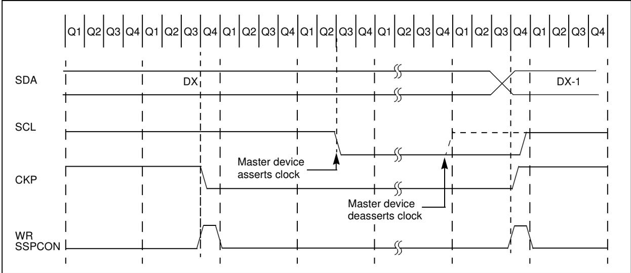
FIGURE 9-13: I<sup>2</sup>C SLAVE MODE TIMING WITH SEN = 1 (RECEPTION, 7-BIT ADDRESS)
