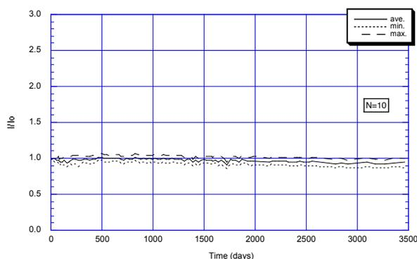
Figure 3 - Typical long term stability of TGS5042
