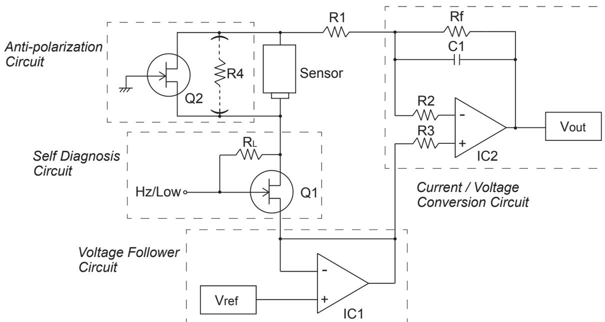
Figure 1 - Example circuit for TGS5xxx sensors
