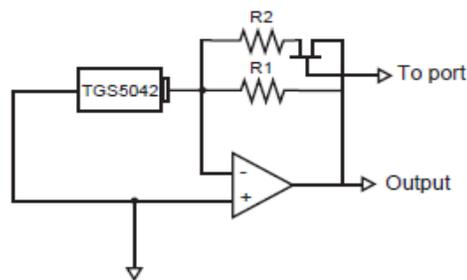
Figure 2 - Circuit for changing gain using a FET
