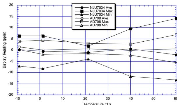
Figure 5 - Temperature dependency of offset voltage for op-amps
