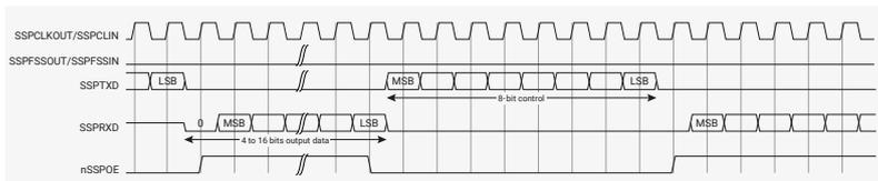
In Microwire mode, the PrimeCell SSP slave samples the first bit of receive data on the rising edge of SSPCLKIN after SSPFSSIN has gone LOW. Masters that drive a free-running SSPCKLIN must ensure that the SSPFSSIN signal has sufficient setup and hold margins with respect to the rising edge of SSPCLKIN.
