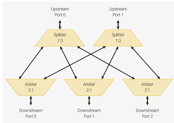
The crossbar is built from two components:
