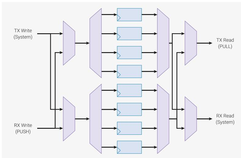
Another example is a UART: because the TX/CTS and RX/RTS parts of a UART are asynchronous, they are implemented on two separate state machines. It would be wasteful to leave half of each state machine's FIFO resources idle. The ability to join the two halves into just a TX FIFO for the TX/CTS state machine, or just an RX FIFO in the case of the RX/RTS state machine, allows full utilisation. A UART equipped with an 8-deep FIFO can be left alone for
