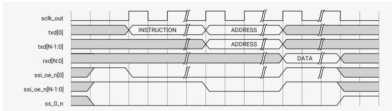
**Case C: Instruction and Address both transmitted in Dual SPI format**
