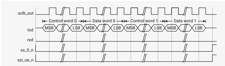
The only modification you need to make to perform a continuous transfer is to write more control and data words into the transmit FIFO buffer, shown in Figure 141. This example shows two data words are written to the external serial slave device.
