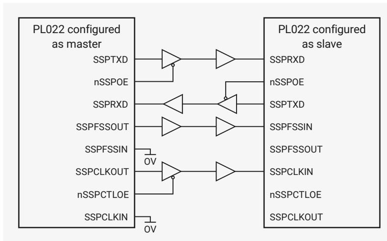
Figure 100 shows how an PrimeCell SSP (PL022), configured as master, interfaces to a Motorola SPI slave. The SPI Slave Select (SS) signal is permanently tied LOW and configures it as a slave. Similar to the above operation, the master can broadcast to the slave through the master PrimeCell SSP SSPTXD line. In response, the slave drives its SPI MISO line onto the SSPRXD line of the master.
