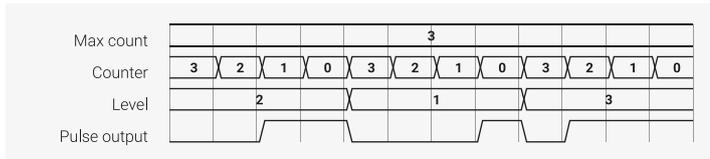
This program repeatedly counts down to 0 with the Y register, whilst comparing the Y count to a pulse width held in the X register. The output is asserted low before counting begins, and asserted high when the value in Y reaches X. Once Y reaches 0, the process repeats, and the output is once more driven low. The fraction of time that the output is high is therefore proportional to the pulse width stored in X.
