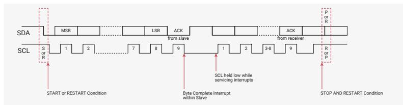
The DW\_apb\_i2c is a synchronous serial interface. The SDA line is a bidirectional signal and changes only while the SCL line is low, except for STOP, START, and RESTART conditions. The output drivers are open-drain or open-collector to perform wire-AND functions on the bus. The maximum number of devices on the bus is limited by only the maximum capacitance specification of 400 pF. Data is transmitted in byte packages.
