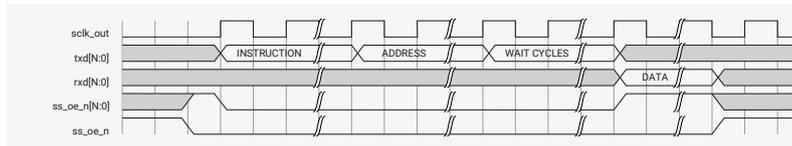
To initiate a dual/quad read operation, CTRLR0.SPI\_FRF must be set to 01/10/11 respectively. This will set the transfer type, now for each read command data will be transferred in the format specified in CTRLR0.SPI\_FRF field.
