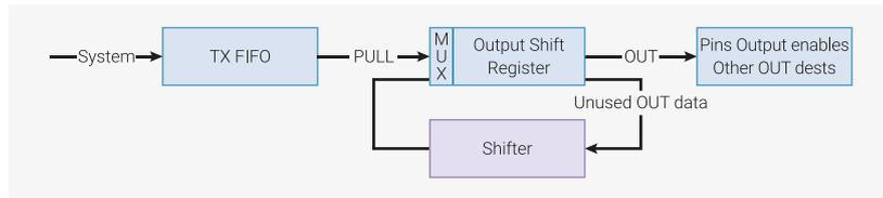
The Output Shift Register (OSR) holds and shifts output data, between the TX FIFO and the pins (or other destinations, such as the scratch registers).
