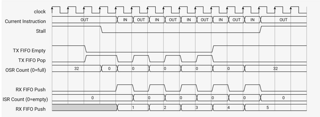
To trigger automatic push or pull at the correct time, the state machine tracks the total shift count of the ISR and OSR, using a pair of saturating 6-bit counters.
