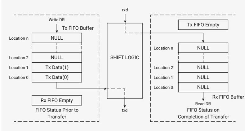
For receive only transfers (transfer mode field (9:8) of the Control Register 0 = 10b), data transmitted from the DW\_apb\_ssi to the external serial device is invalid, so a single dummy word is written into the transmit FIFO to begin the serial transfer. The txd output from the DW\_apb\_ssi is held at a constant logic level for the duration of the serial transfer. Data received from the external serial device into the DW\_apb\_ssi is pushed into the receive FIFO.
