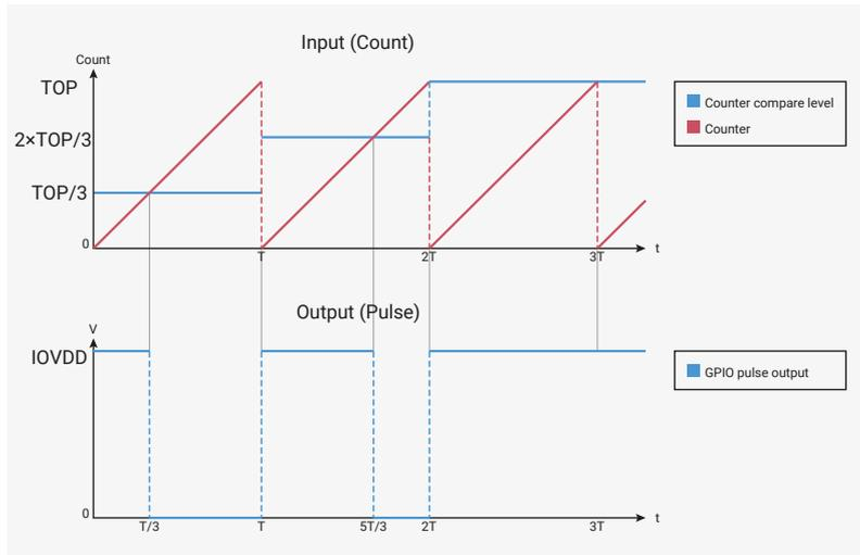
In Figure 108, the input value only changes at the instant where the counter wraps through 0. Figure 109 shows what happens if the input value is allowed to change at any other time: an unwanted glitch is produced at the output.
