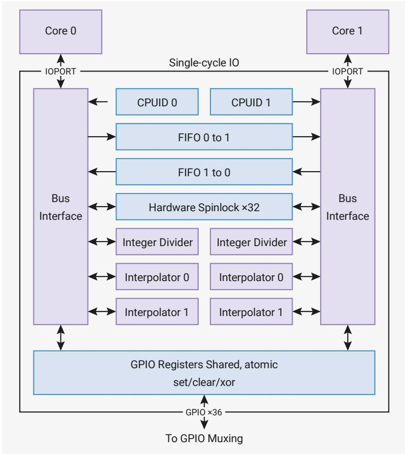
All IOPORT reads and writes (and therefore all SIO accesses) take place in exactly one cycle, unlike the main AHB-Lite system bus, where the Cortex-M0+ requires two cycles for a load or store, and may have to wait longer due to contention from other system bus masters. This is vital for interfaces such as GPIO, which have tight timing requirements.
