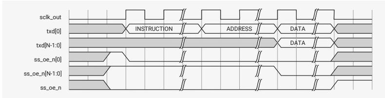
**Case B: Instruction transmitted in standard and address transmitted in Enhanced SPI format**
