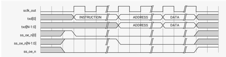
**Case C: Instruction and Address both transmitted in Enhanced SPI format**
