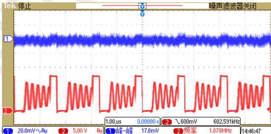
PWM MODE (CH1:V<sub>OUT</sub>(ripple) CH2:V<sub>sw</sub>)
