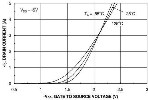
Figure 15. Transfer Characteristics.
