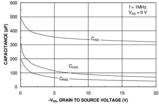
Figure 18. Capacitance Characteristics.
