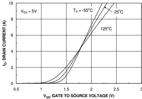
Figure 5. Transfer Characteristics.
