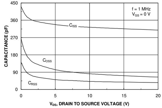
Figure 8. Capacitance Characteristics.
