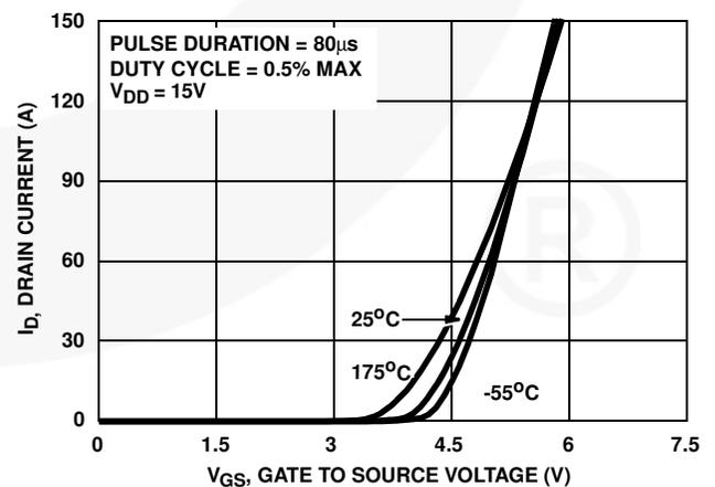
FIGURE 8. TRANSFER CHARACTERISTICS
