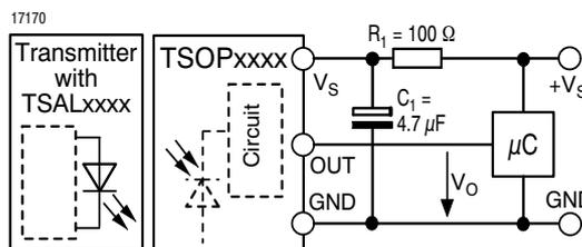
$R_1 + C_1$  recommended to suppress power supply disturbances.
