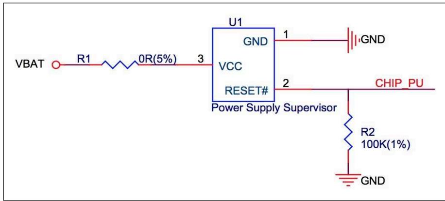
Figure 6: Reset Circuit
