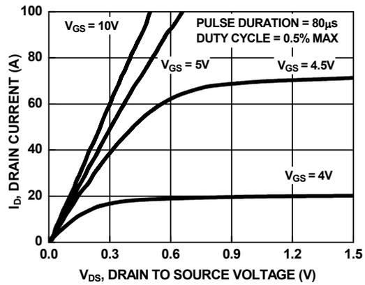
Figure 8. Saturation Characteristics
